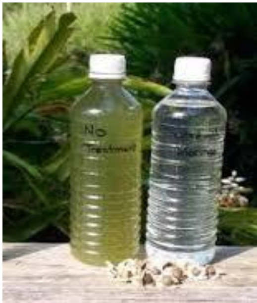
Figure 5: Moringa for purification of turbid water (before and after treatment) (Lea, 2010).
