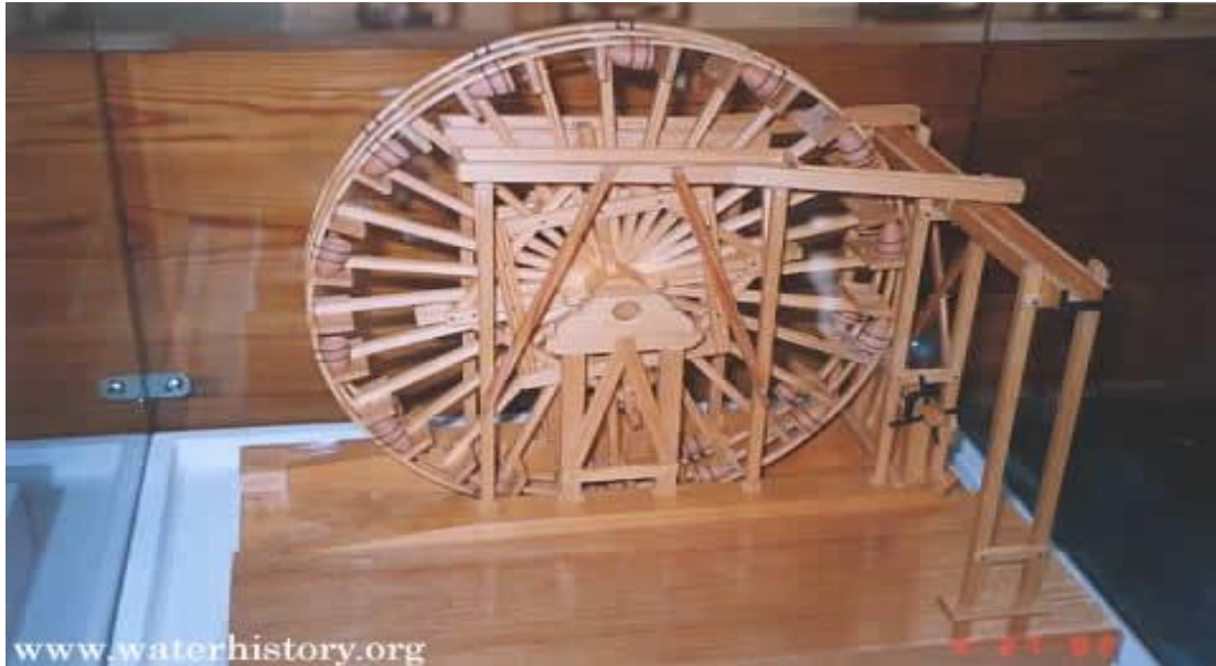
Figure 2.3: A noria, buckets attached to a waterwheel, was another device used to lift water.
