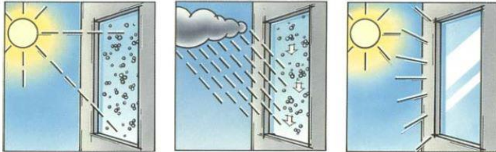
Figure 6. ‘Photo-induced hydrophilicity and self-cleaning property of a \text{TiO}_2 -coated surface’ (28: p.19).
