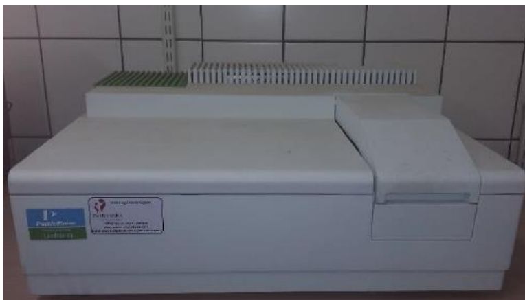
Figure 25. Photograph of the Perkin-Elmer Lambda 35 UV/Vis spectrophotometer.
