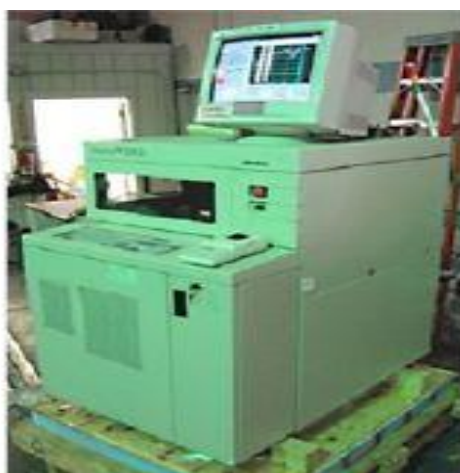
Figure 24. A photograph of a Sloan DEKTA3 profilometer.
