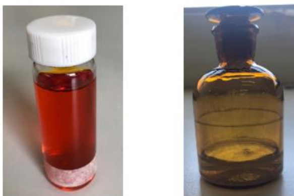
Figure 27. Photograph of a 0.4mmol/g TiO_2 (left) and 0.8mmol/g Ag-NPs (right) precursor solutions.
