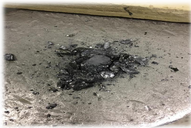
Figure 6: Brittle button (the button breaks into scattered pieces once hammered).
