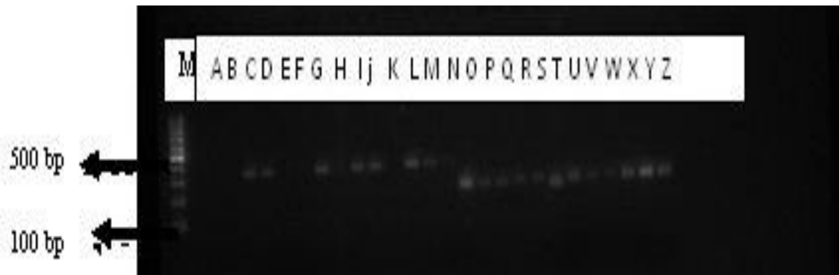
Figure 8: PCR products for lactic acid bacteria separated using gel electrophoresis on a 2% agarose gel. M: 100bp DNA ladder, lane C,D,G,H,I,J,L,M and N (Ec338f-Ec518r primer), O,P,Q,R,S,T,U,V,W,X,Y,Z (WBAC1-WBAC2 primer).
