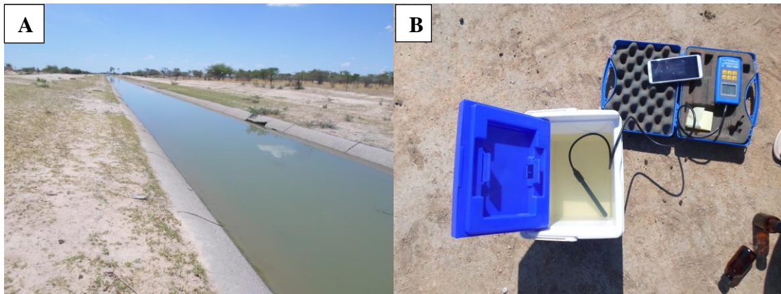
Figure 3: A. The Calueque-Oshakati canal, B. the on-site measurement of water temperature and electric conductivity.
