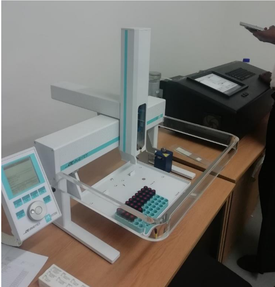
Figure 5: An automated liquid-water analyser performing the stable isotope composition analysis.
