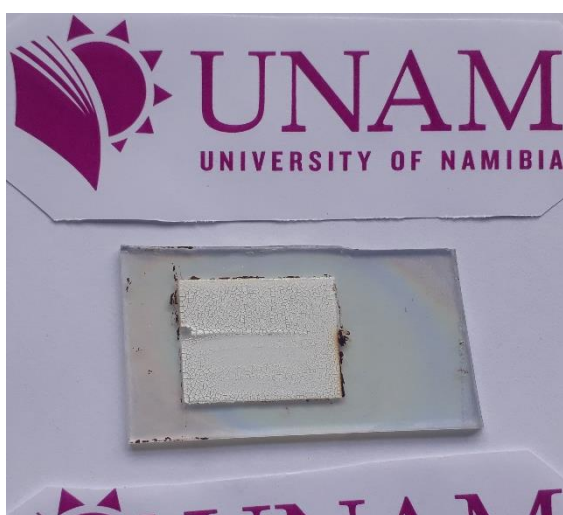
Figure 19 Fabricated Titanium dioxide paste FTO glass substrate after air drying.
