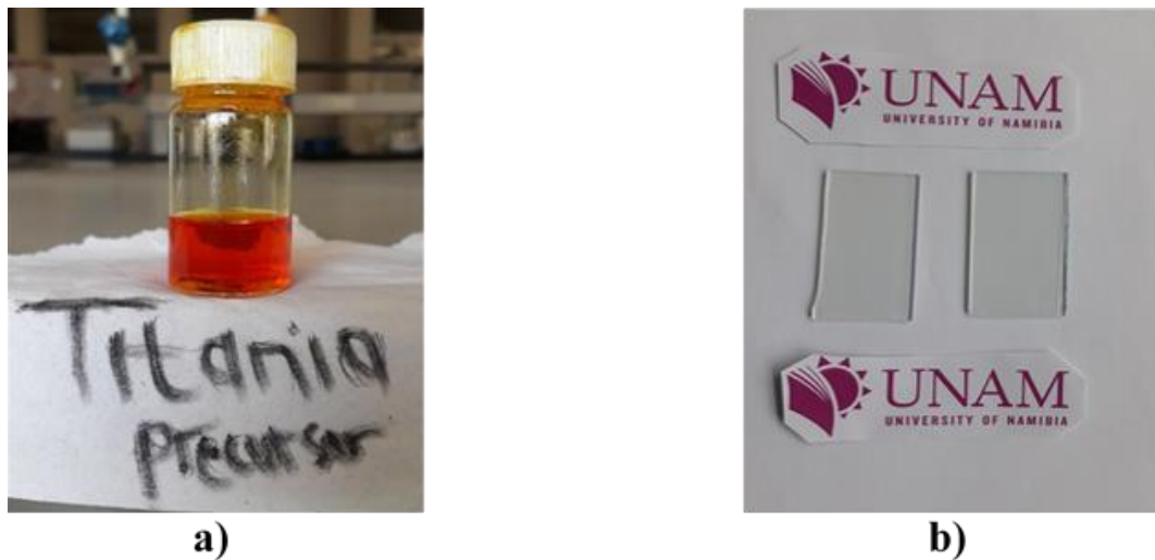
Figure 17 a) Titania precursor solution ( \text{TiO}_2 ), and b) fabricated \text{TiO}_2 thin film.
