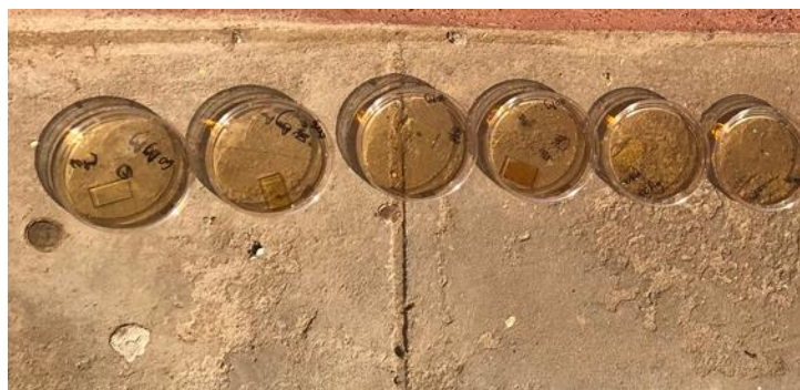
Figure 28: Decomposition of MO under visible light
