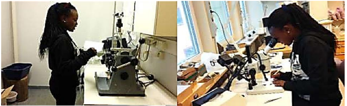
Figure 3-2: The panned samples were taken to the FRANTZ machine to separate the magnetic material from the non-magnetic material. b) Sample after going through the FRANTZ are then hand-picked under the binocular microscope from the glass plates and placed on a separate glass plate.
