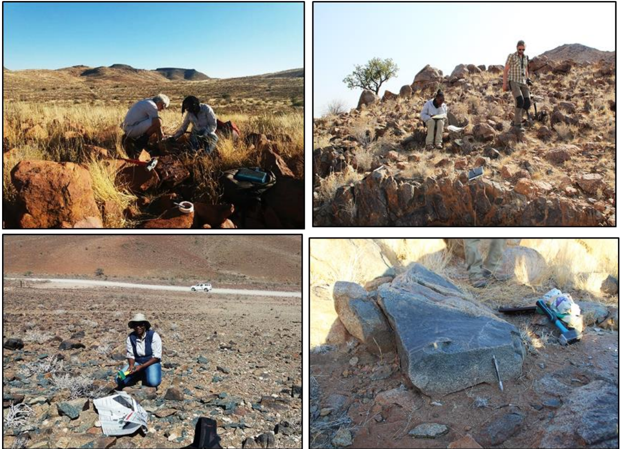
Figure 3-1: Field images while collecting samples from the Barby Formation, South-west of Helmeringhausen. The images show the various tools used while sampling such as hammer, newspaper, cello tape, notebook and GPS
