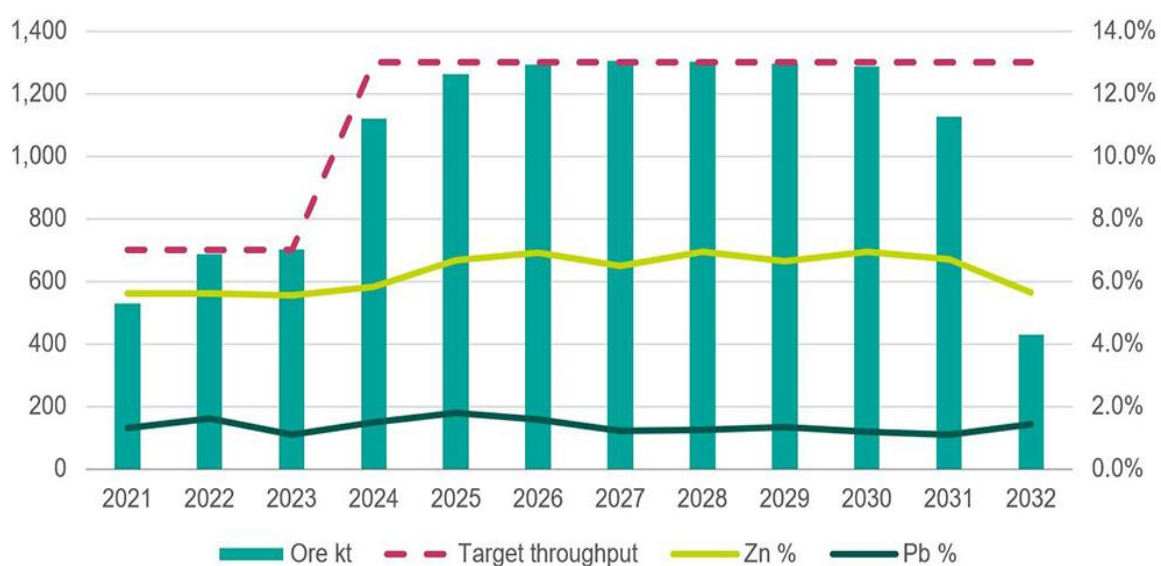
Figure 65: An expected increase in annual ore production due to Rosh Pinah Expansion "RP2.0". Source: (Trevali, 2022).
