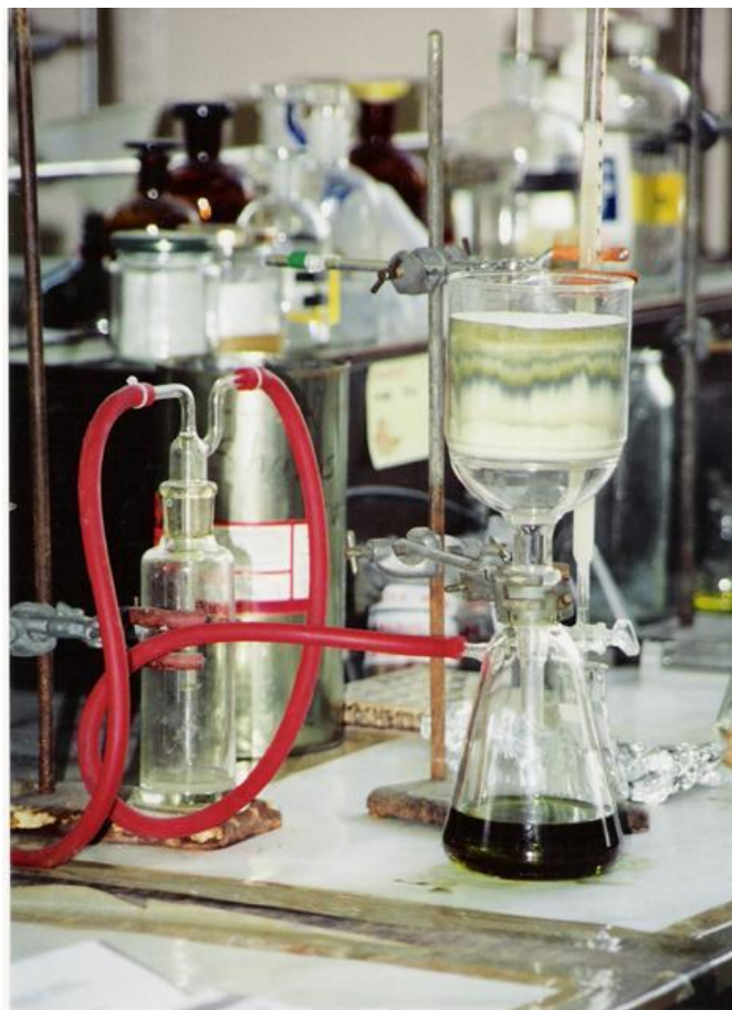
Figure 8: Experimental setup for vacuum liquid chromatography (VLC) [65].
