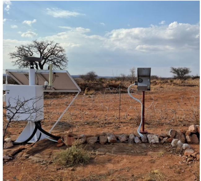
Figure 1. GNSS station (left, in white) installed in 2022 and 210 GHz WVR (right) installed in 2024 to validate GNSS PWV data at the H.E.S.S. site.
