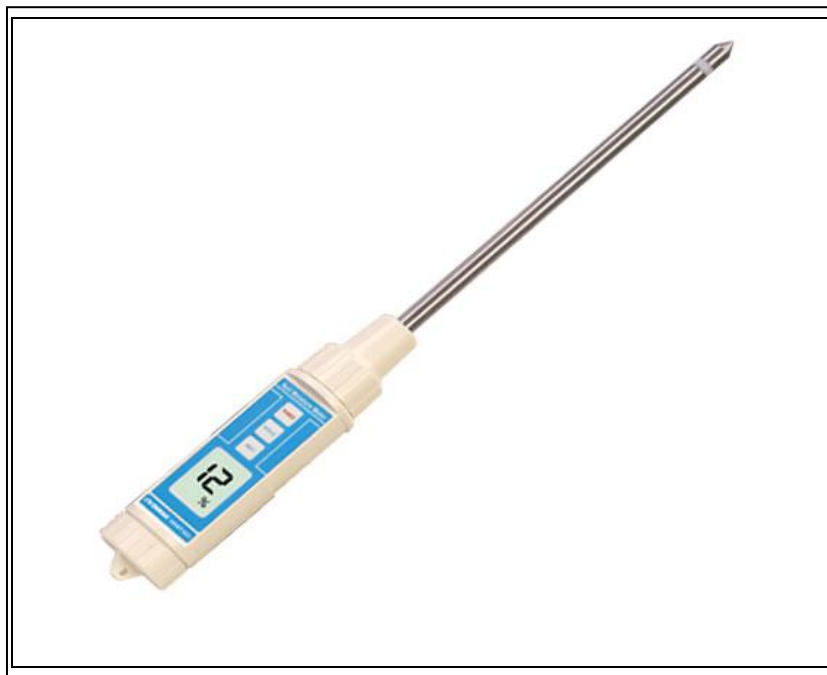
Figure 12: A HSM50 Precision Digital Soil Moisture Meter used at Ogongo experimental site
