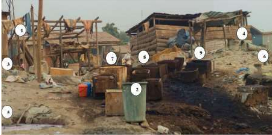
Figure 4. Tannery site in Ashanti Region, Ghana, Africa. 1. Curing (drying); 2. Soaking; 3. Liming; 4. Unhairing; 5. Bating; 6. Fleshing; 7. Vegetable tanning; 8. Red dyeing; 9. Black dyeing. Photo:
