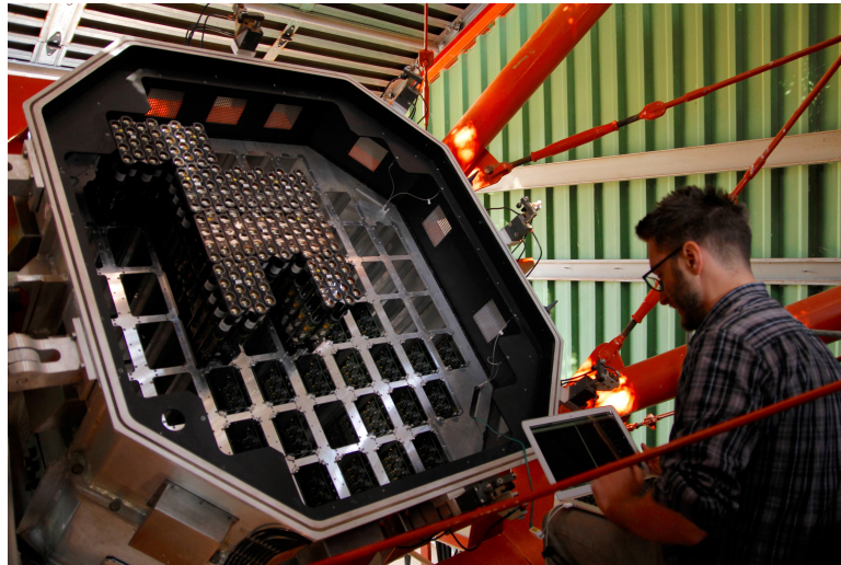
Figure 3.2. The view of the front part of CT1 camera during the upgrade in 2015. When fully complete, this front part of the camera contains 60 interchangeable drawers, each with 16 PMTs lodged in a pigeon-hole plate.
