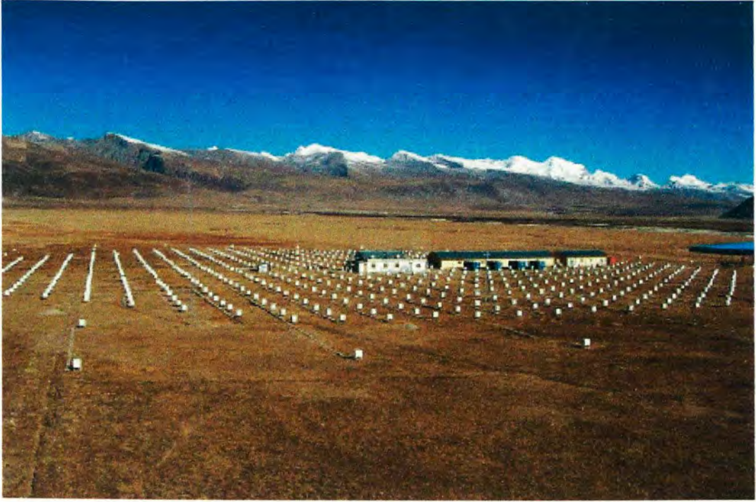
Figure 3.3: Air shower array in Yangbajing Tibet, composed of 1848 detector elements [43]. Figure from [44].
