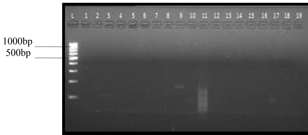
Figure 13: Primer MARA 067 a typical microsatellite locus that could not be scored or did not give any amplification. Sample 1-19 are individuals from Omitara, lane L contains a 100 bp ladder and the gel was 2.5 %. Electrophoresis was at 100 V for 1 hour.
