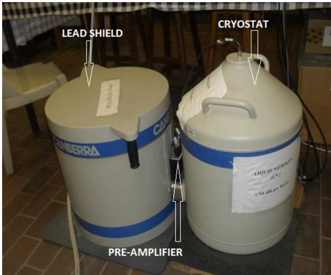
Figure 3.10 Lead shield and Cryostat
