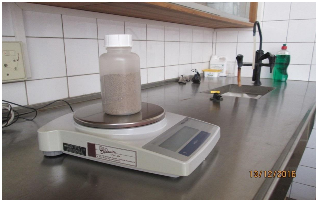
Figure 3.7 Determination of the weight of a soil sample using an electronic scale.
