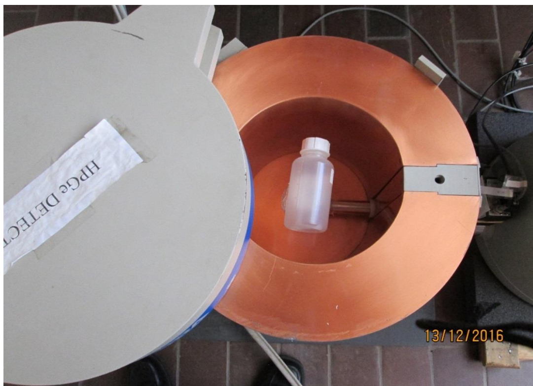
Figure 3.16 HPGe Detector with empty bottle ready for background counting
