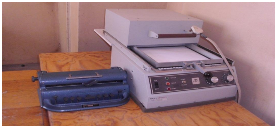
Figure 4.14: The Perkin braille and the thermoform machines
