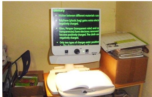
Figure 4.17: A closed-circuit television (CCTV)
