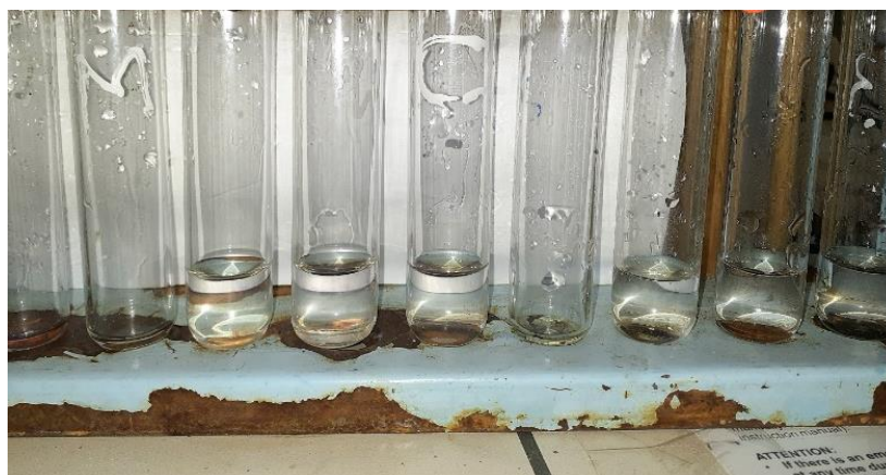
Figure 3.18. Iron test done on Grundorn's groundwater.
