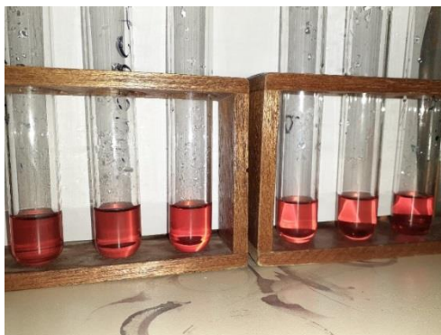
Figure 3.21. Carbonate hardness test done on Nico's bucket filtered water.
