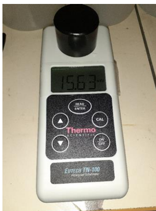
Figure 3.17. The portable turbidity meter used in the study.
