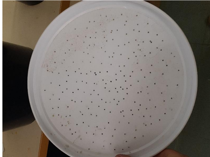
Figure 2.4. Diffuser plate made with a drill.
