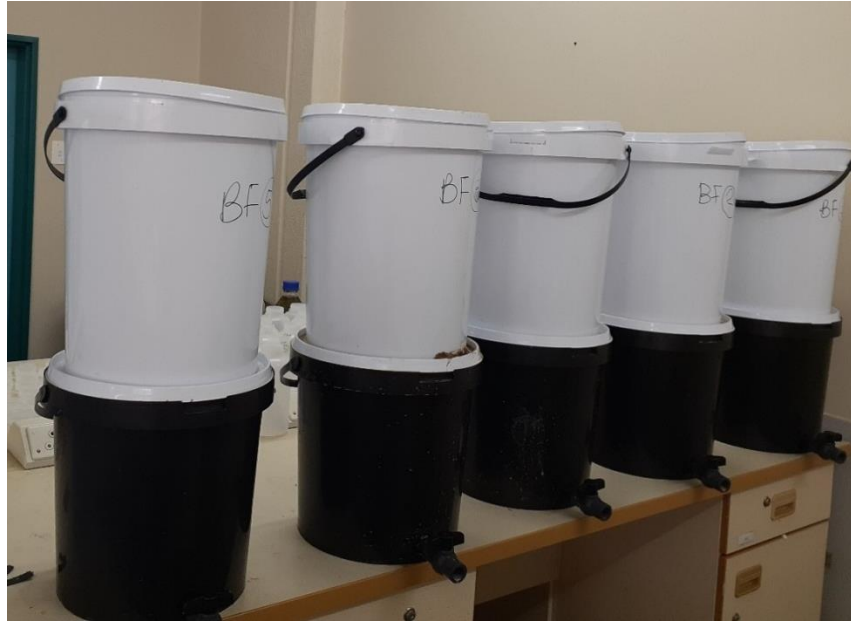
Figure 3.24. All bucket filters during filtering.
