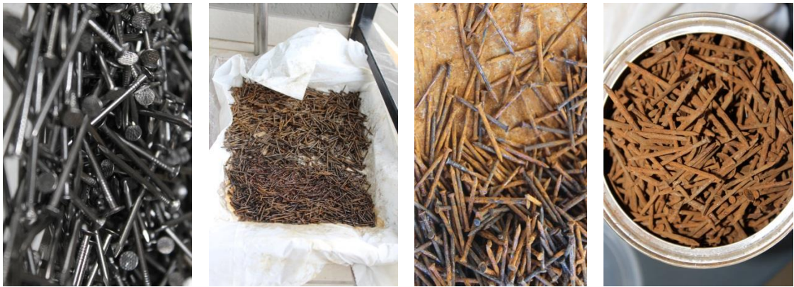
Figure 22 – Nail rusting process. Photographs: By Author
