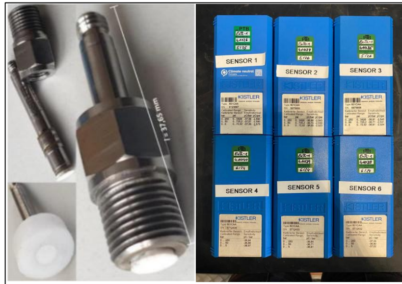
Figure 11: Kistler 601CAA pressure sensors with 1mm RTV silicone.
