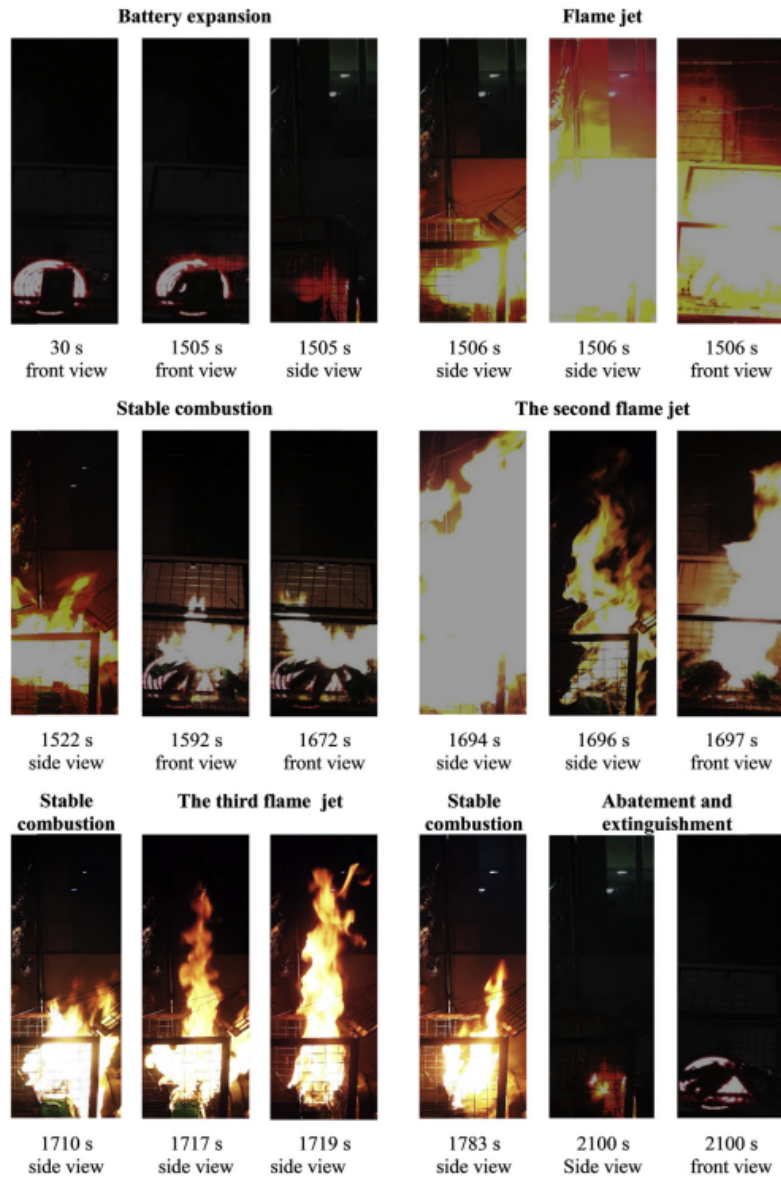
Figure 2. The combustion process in the 100% SOC battery’s full-scale burning tests. (With permission from author). This images show different stages of thermal runaway, including: battery expansion (30s - 1505s), jet flames (1506s), stable combustion (1522s – 1672s), second jet flame (1694s – 1697s), third jet flame (1710s – 1719s), stable combustion (1783s) and lastly the abatement and extinguishing at 2100s [31].
