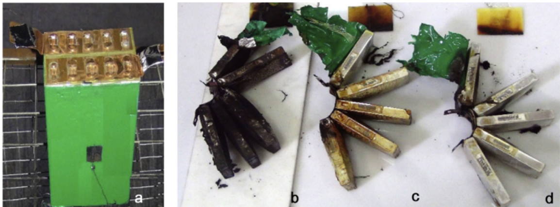
Figure 3. (a) 50 Ah LiFePO 4 /graphite battery before the full-scale burning test; (b) 100% SOC, (c) 50% SOC and (d) 0% SOC batteries after full-scale burning tests. (With permission from author) [31].
