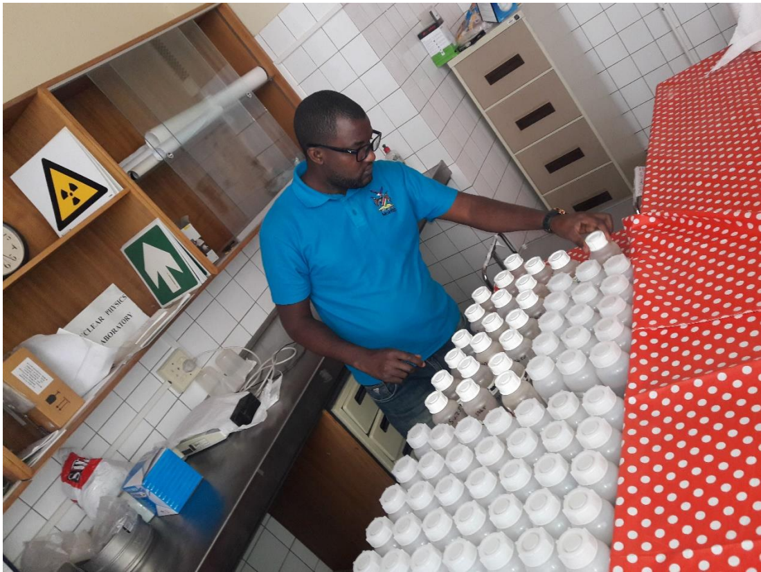
Figure 3.8: Soil samples stored in the laboratory for radioactive equilibrium prior to radio-analysis
