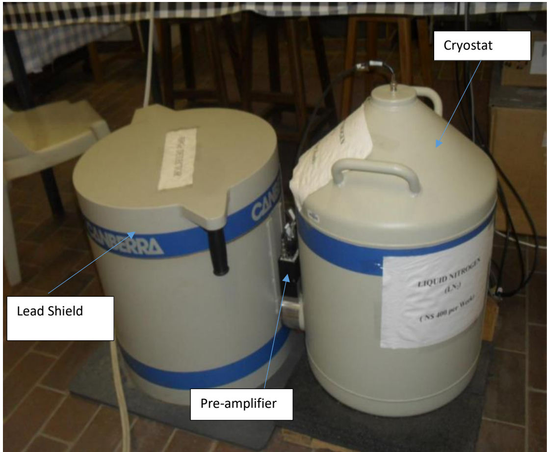
Figure 3.10: A Model 7915-30 Cryostat for supplying LN2 to the HPGe detector inside a Canberra Model 737 lead shield
