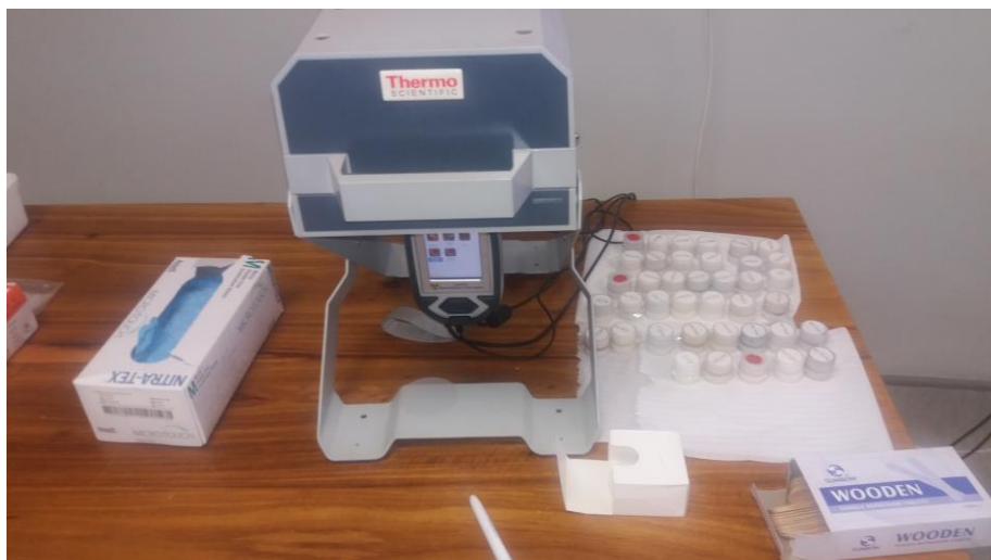
Figure 3.3.2: Sample holders containing the pulp samples ready for analysis (red labeled samples are standards).
