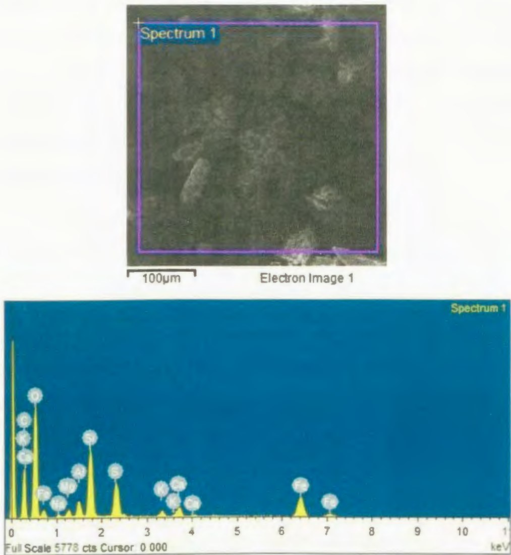
Figure 4-4: Backscattered electron image (up) with EDS (down) of the raw tailings sample
