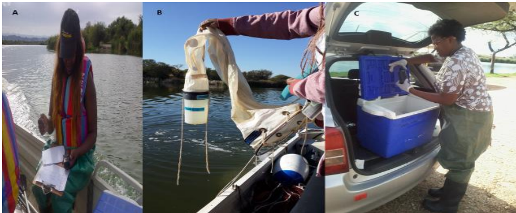
Figure 22: Sampling Procedure. (A) Site data on log book, (B) 63µm phytoplankton net for microalgae sampling, (C) Storing sample bottles in a cooler box for analysis.
