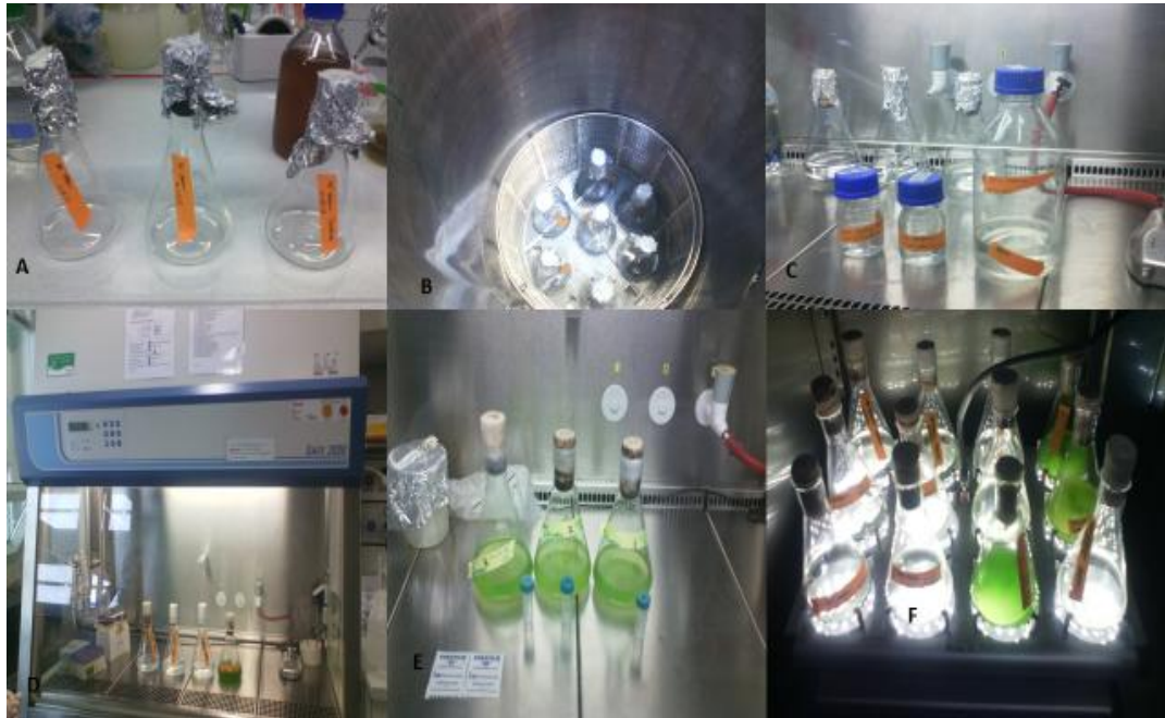
Figure 25: Experimental set up for pre-cultures. (A) Empty 500 mL Erlenmeyer Flasks with cellulose stoppers and aluminum foil, (B) Autoclaving Empty 500 mL Erlenmeyer Flasks with cellulose stoppers and aluminum foil, (C) BG 11 0 medium and two (NaHCO 3 and HEPES) buffer stock solutions under the Thermo Scientific Biological Safety Cabinet, (D) Inoculation of 3 Erlenmeyer Flasks to an Optical Density (OD) of 0.1 at 750 nm, (E) 500 mL Erlenmeyer Flasks covered with Parafilm, (F) Erlenmeyer Flasks set on permanent illumination of 180 \mu\text{mol}/\text{m}^2/\text{s} (LED) at room temperature of 25 \pm 1 °C, agitated at 100 rpm for 14 days.
