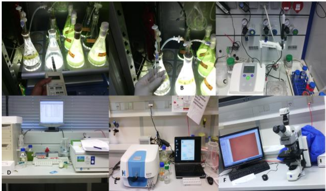
Figure 26: Monitoring instruments. (A) Measuring Light intensity using a quantum meter (Model LI 250 light meter), (B) Sampling via Braun Leur Lock Omnifix syringe via Straight Male threaded swabable valve, (C) Measuring pH via Mettler Toledo, (D) Perkin Elmer Lambda 35 ES UV/VIS Spectrophotometer for measuring Optical Density, (E) Flow-cytometry via Guava easyCyte for measuring cell concentrations, (F) Bio-AG Zeiss Axioscope A.1 for microscopy.
