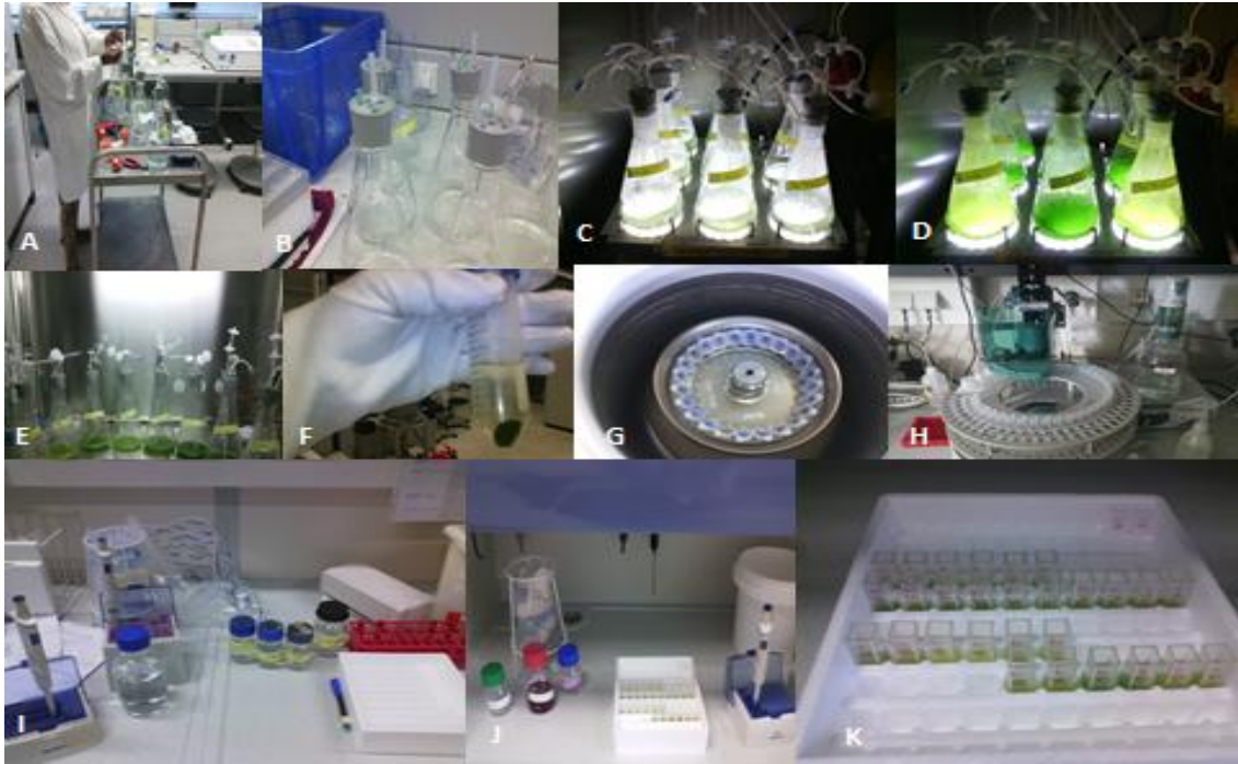
Figure 30: Main-culture set up and procedure. (A & B) Make shift main-culture bioreactors, (C & D) Aeration and inoculation of main-cultures, (E, F, G & H) Centrifugation for BDM and Ion Chromatography, (I) Medium for lipid analysis (J & K) DMSO and Nile red method.
