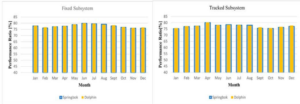
Figure 4. 5: Springbok and Dolphin site comparative simulation results, of performance ratio (PR), With Storage
