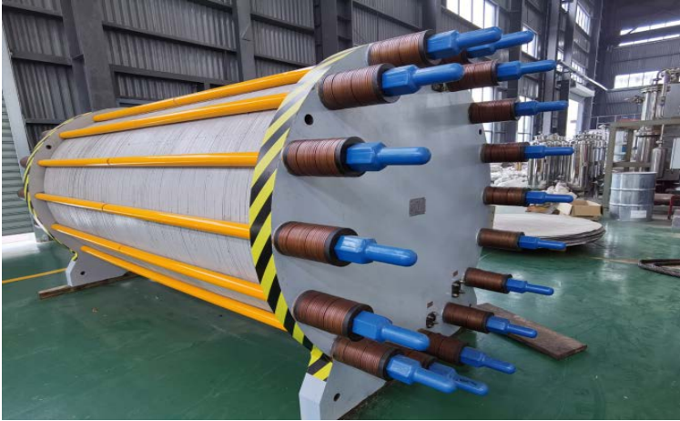
Figure 3. 7: : Photo of the DQ1000 Alkaline Electrolyser
