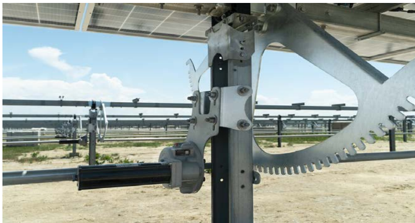
Figure 3. 8: Ideematec Horizon L: TEC 1P tracker, sourced from [103]
