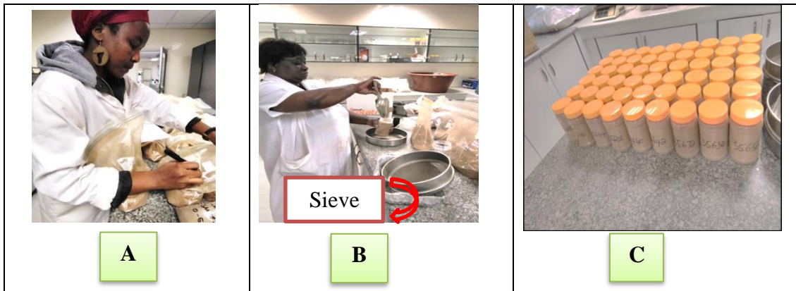
Figure 9: (A) Sorting and labelling (lab codes) (B) Sieving and bottling the soil samples; and (C) soil samples ready for analysis
