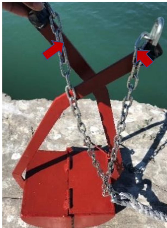
Figure 3.26 shows the mechanism of how to open the sediment grab.
