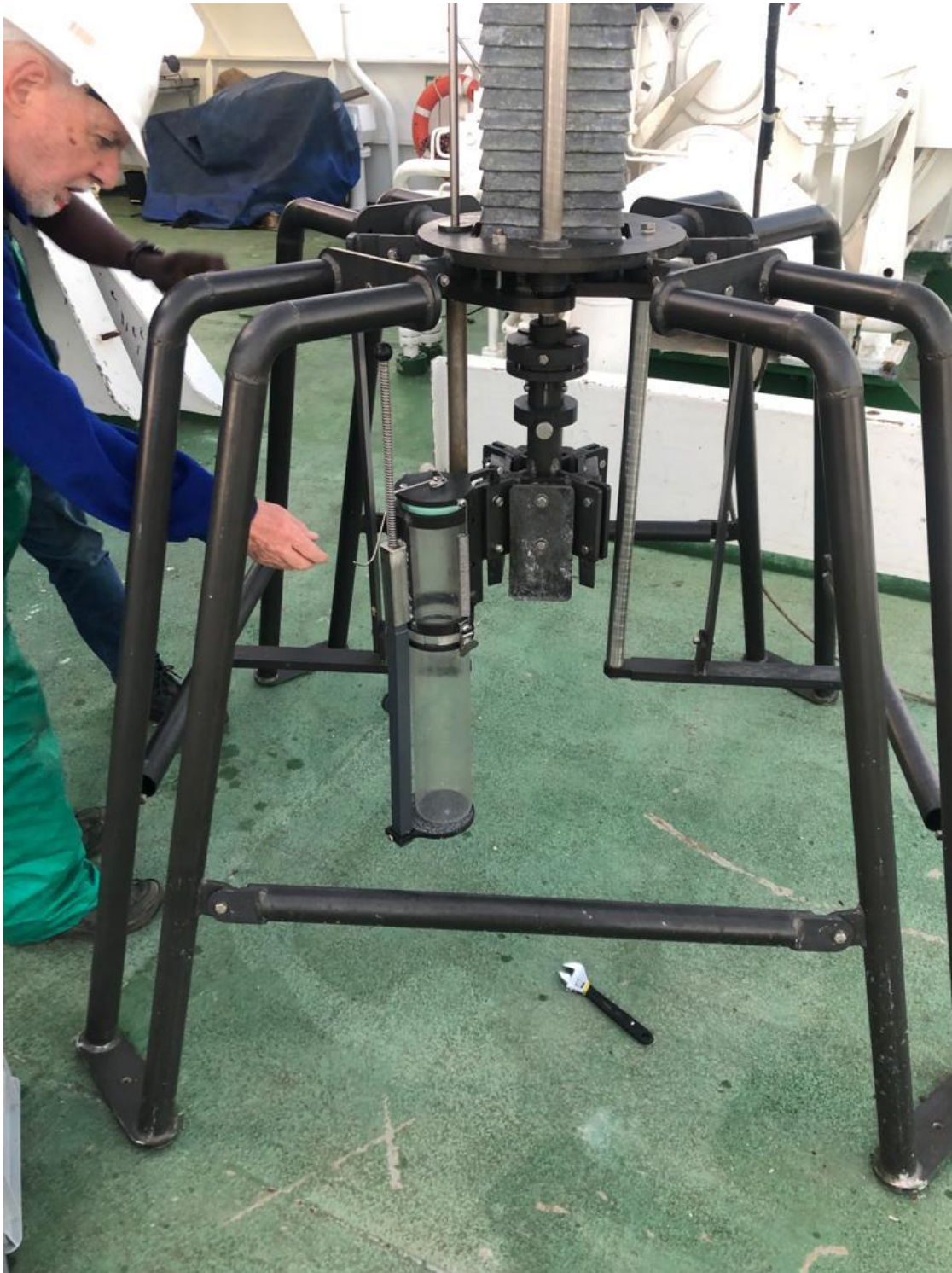
Figure 3.29 shows Kurt Hanselmann (Emeritus Professor of biogeochemistry) pointing towards the multi-corer on the deck with the core tube.
