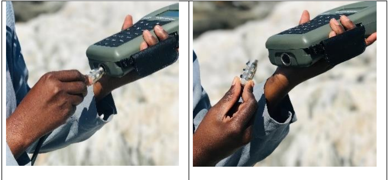
Figure 3.8 show the connection of the probe cord (the metallic part) to the meter.
