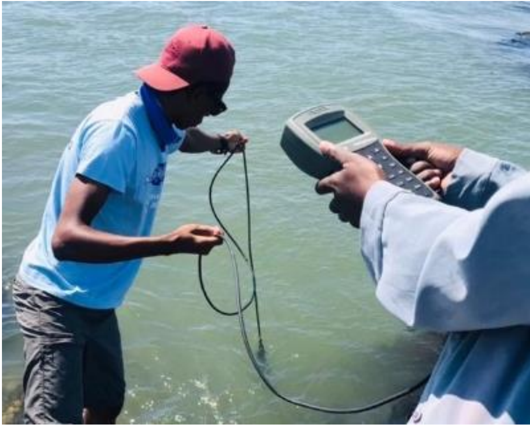
Figure 3.14 shows Loyiso with Iriya from Kelp Blue using the multiparameter sonde to take the water geochemistry reading at the coastal area.
