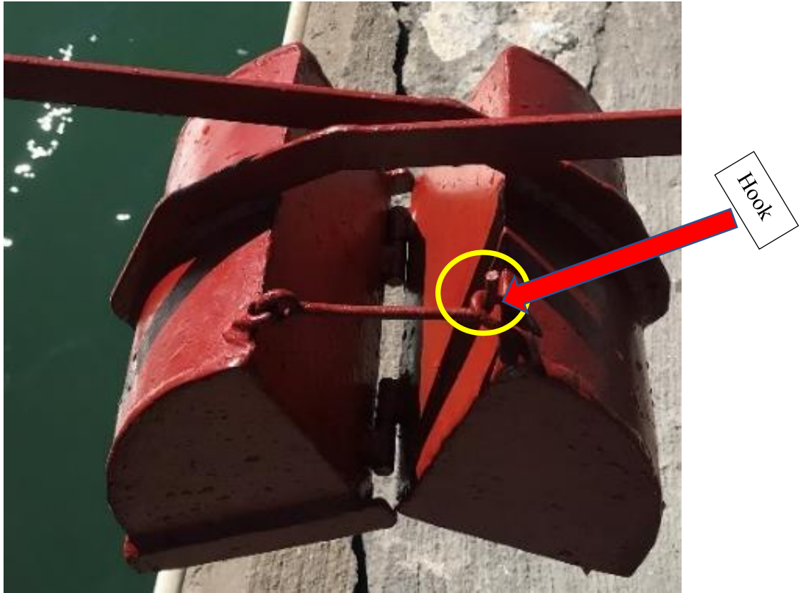
Figure 3.27 shows how to connect the hook to the open slit of the grab.
