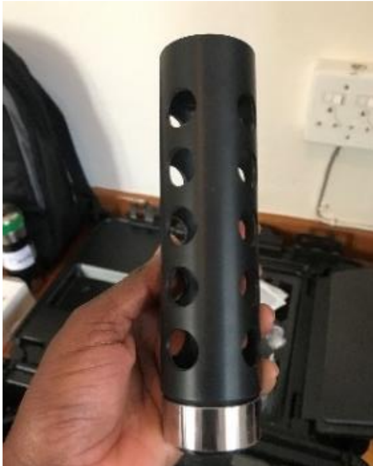
Figure 3.11 shows long shield cover for probes used when deploying the probe in the water.
