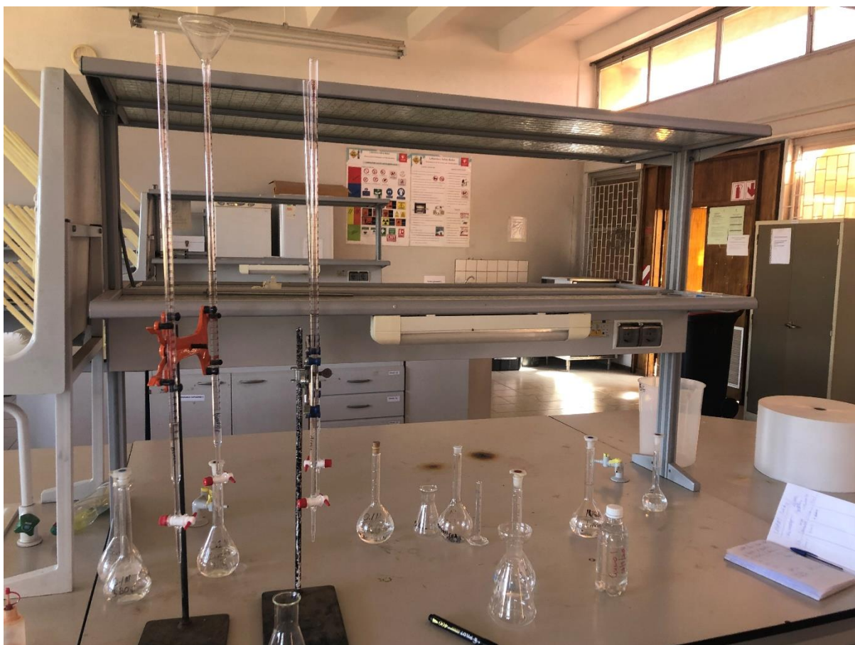
Figure 3.23 shows the burette set up for titration in the UNAM organic chemistry lab with volumetric flask contain different prepared titrants.
