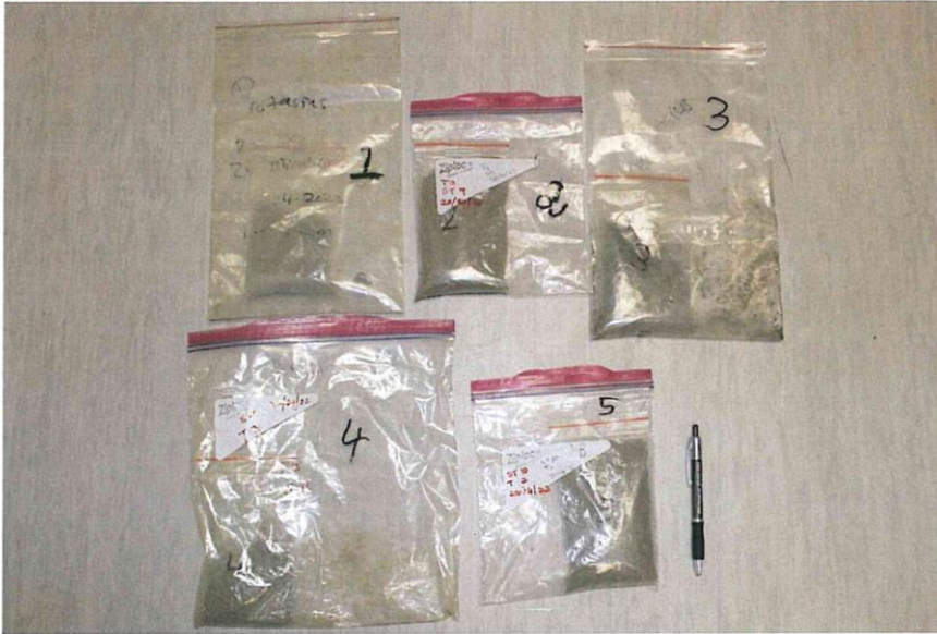
Fig. 1: Submitted samples; Sample No. 1 (mass: 26 g), Sample No. 2 (mass: 224 g), Sample No. 3 (mass: 64 g), Sample No. 4 (mass: 70 g), and Sample No. 5 (mass: 354 g).
