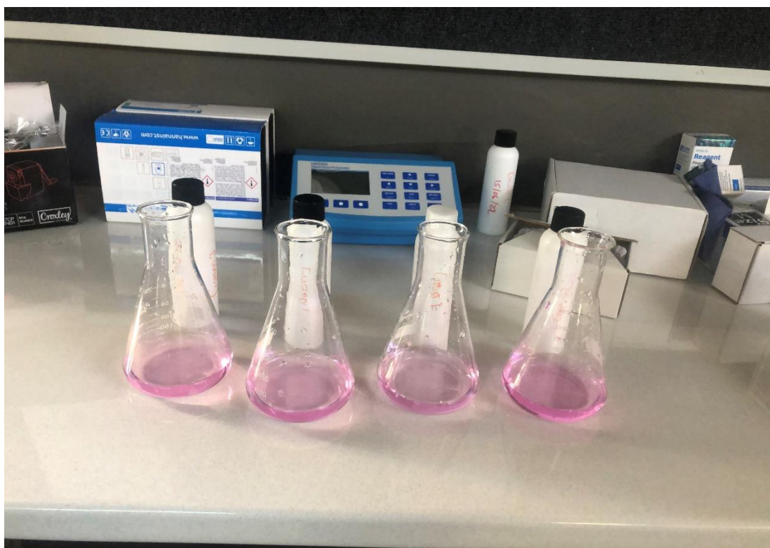
Figure 3.25 shows the endpoint reaction of the analyte (seawater sample) and titrants.
