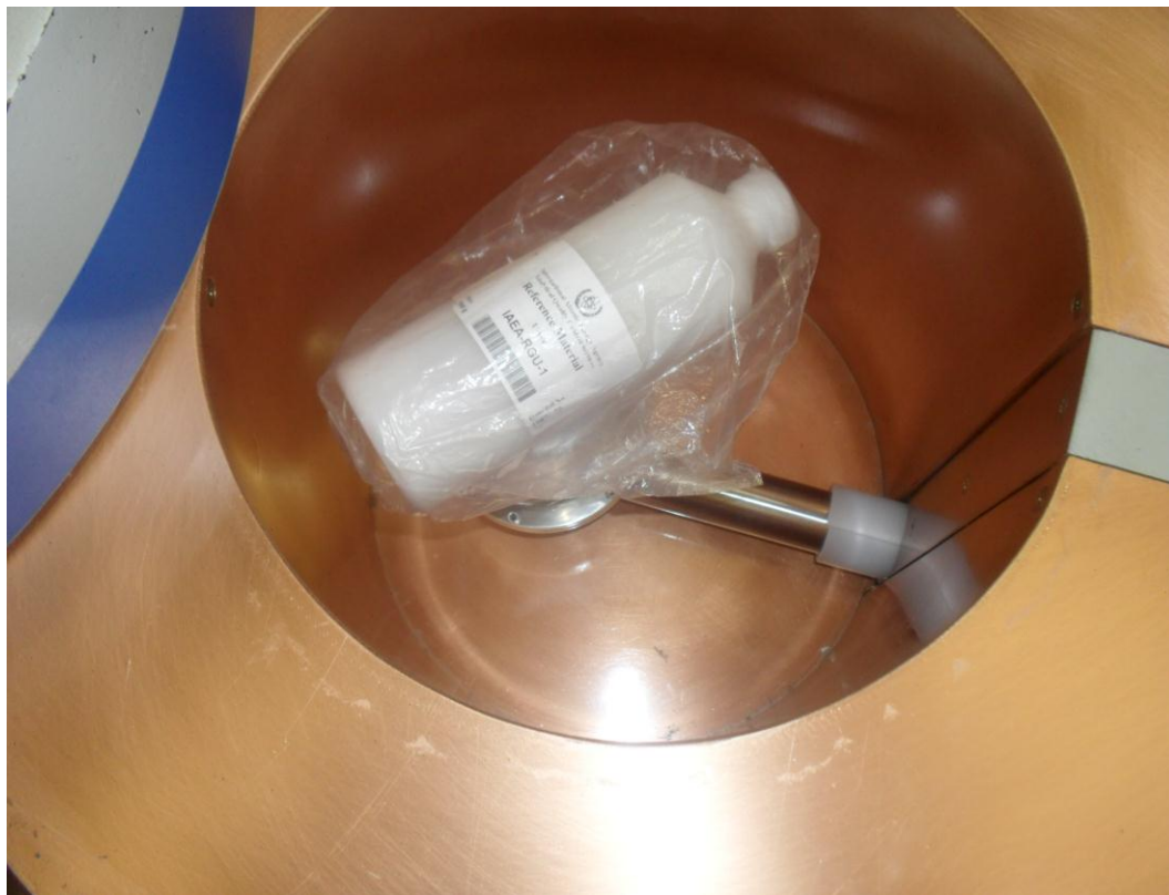
Figure 4.13: Reference material (RGU-1) placed on the HPGe detector inside a lead shield.
