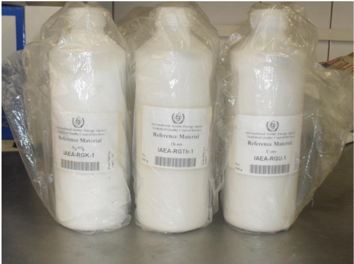
Figure 4.8: Photograph of IAEA reference materials RGU-1, RGTh-1 and RGK-1.
