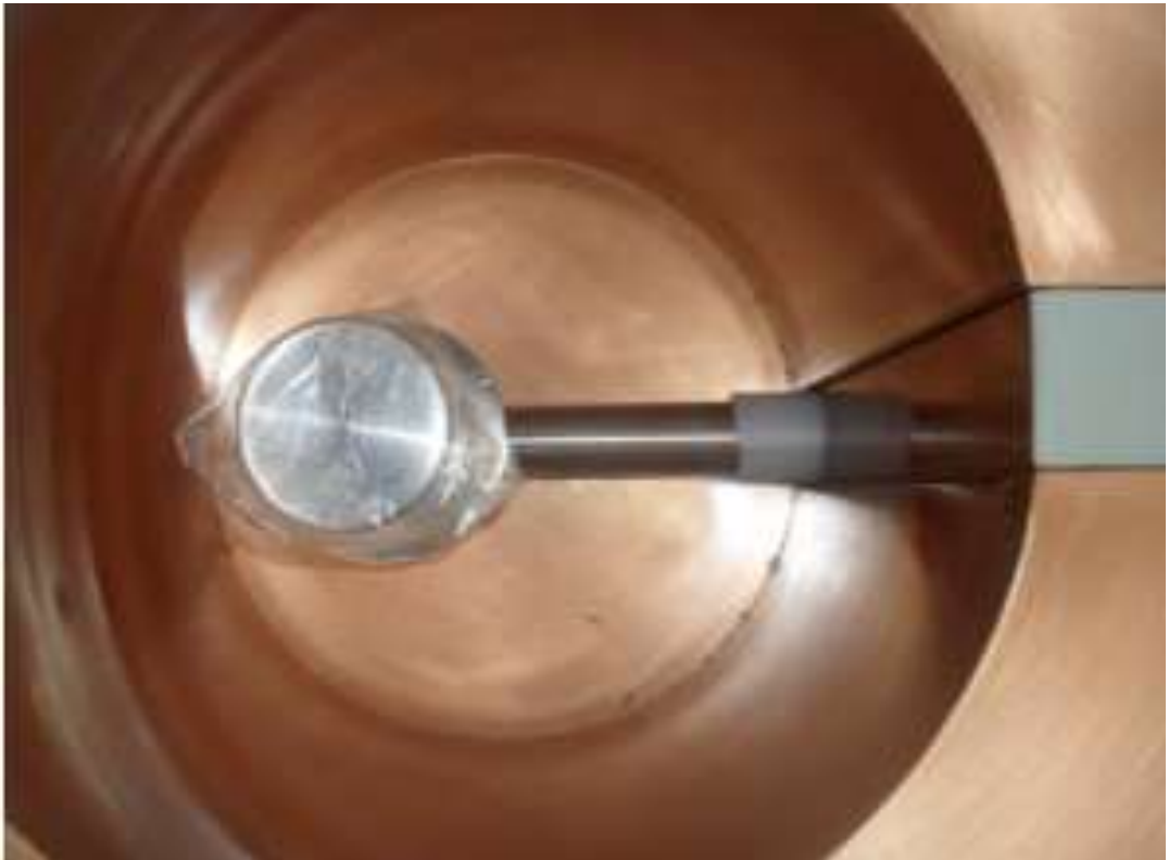
Figure 3.6: HPGe detector in a Lead shield
