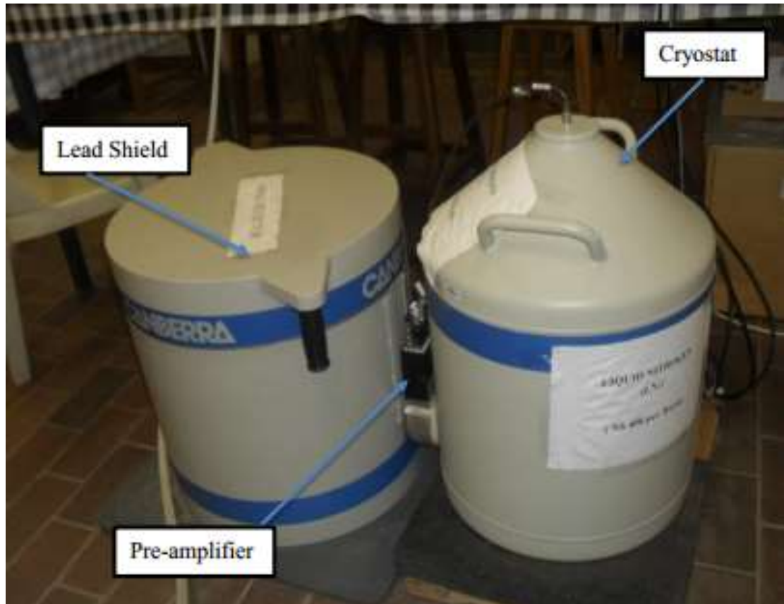
Figure 3.7: Lead shield and Cryostat
