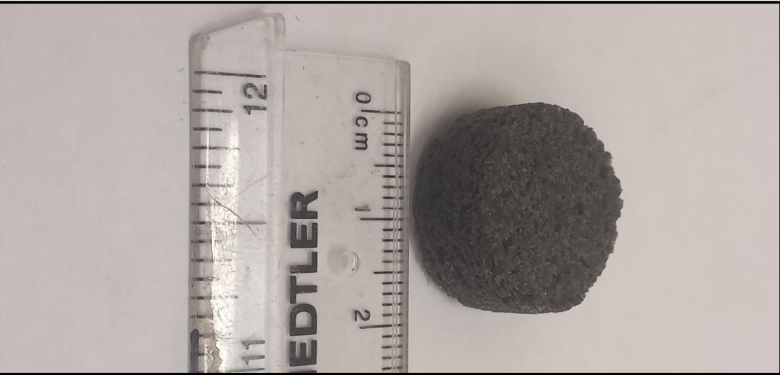
Figure A-12: 20mm diameter maintained after sacrificial porogen removal.
