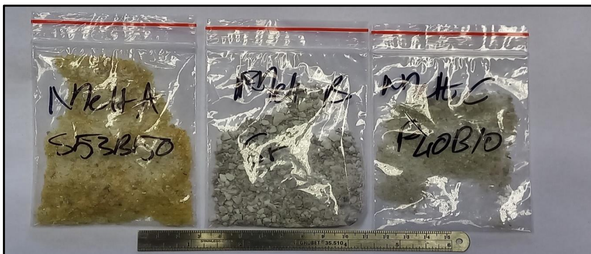
Figure A-8: Crushed glasses for planetary ball mill charge.
