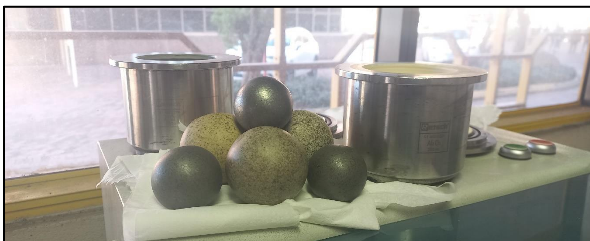
Figure A-9: Zirconium lined milling jars and milling balls for pulverizing.
