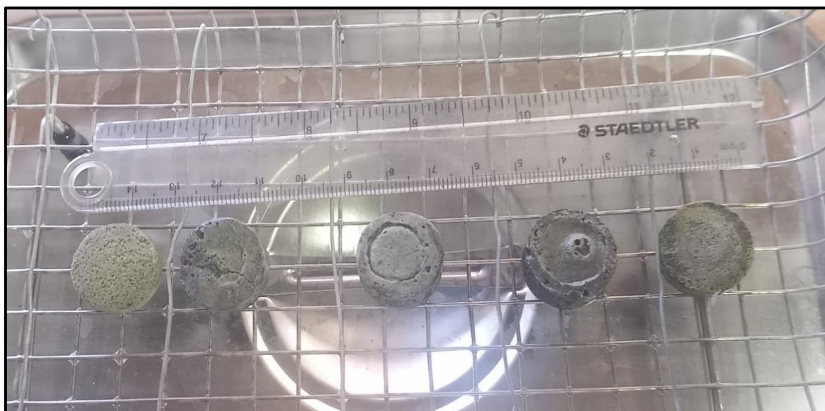
Figure 4-16: Porous Scaffolds After Ultrasonic Cleaning and NaCl leaching.
