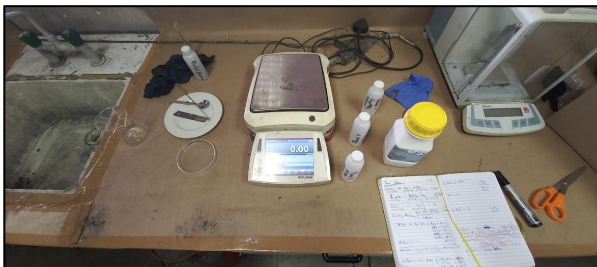
Figure A-2: Reagent measuring and batching with a top pan balance.
