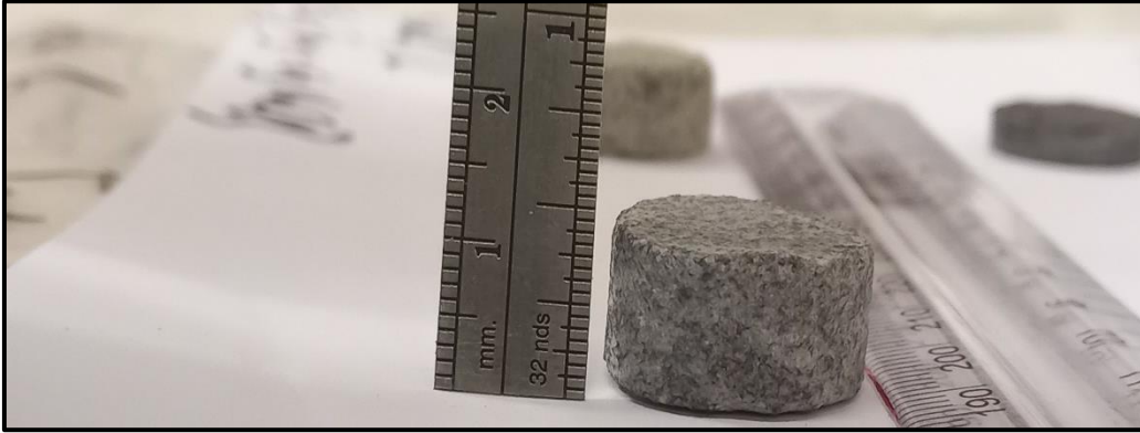
Figure 4-14: S53B50 Sintered Specimen before NaCl Porogen Removal by Salt Leaching.
