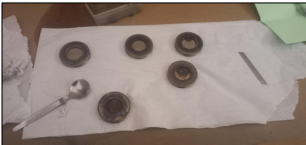
Figure A-10: X-ray diffraction powder sample preparation.
