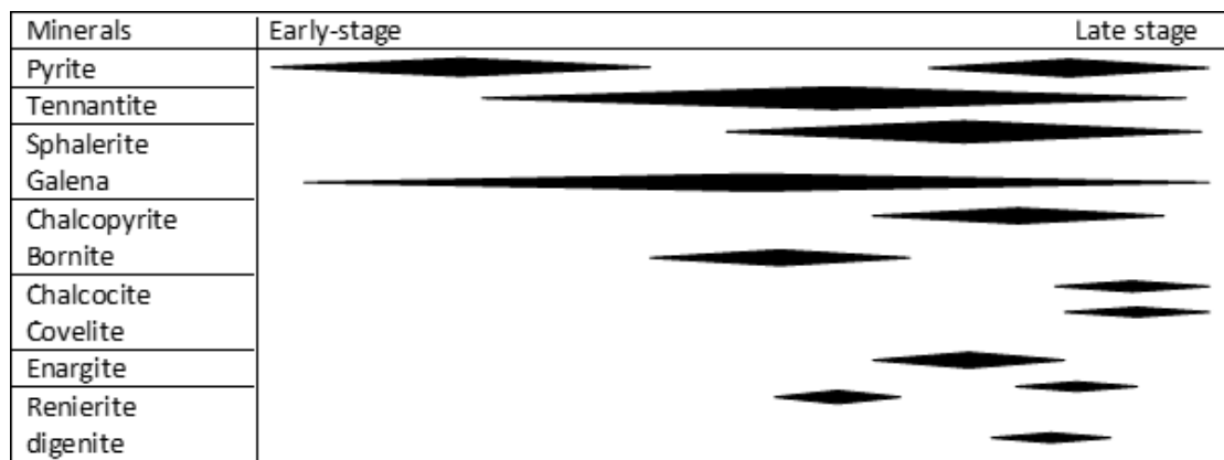
Fig. 6.7-1 Paragenetic sequence of sulfide minerals in the Tsumeb deposit samples from Level 16, 17, 18, 19, 20, 29, 30, 32, and 46
