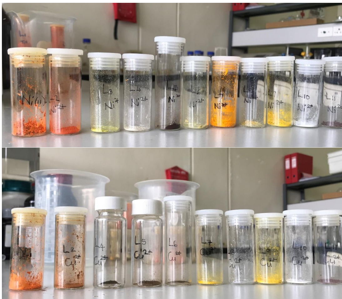
Figure 33. Ligands and metal complexes with varying colours, that were synthesized in the present study. The names of the compounds are indicated on the vials.
