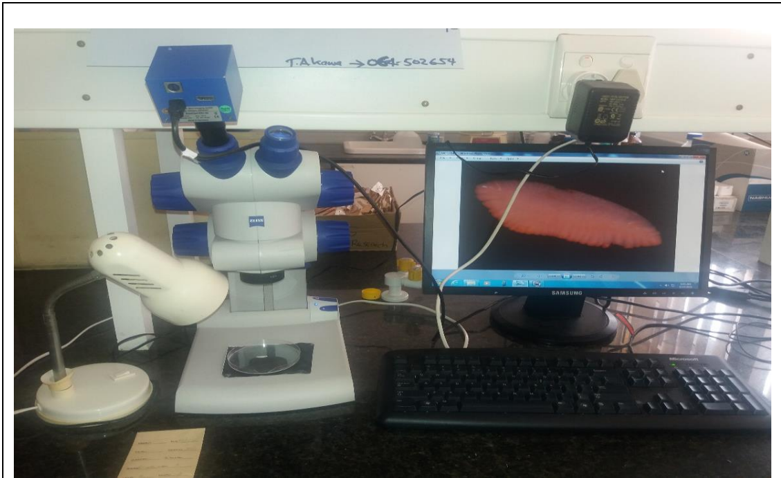
Figure A1: Laboratory set up for taking M. capensis otolith images using a Zeiss Stemi DV4 Stereotype microscope embedded with a Zeiss Axio-camera.
