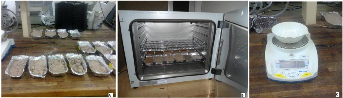
Figure 11. Soil samples in trays (A), soil samples in the oven (B) and soil sample being weight (C).
