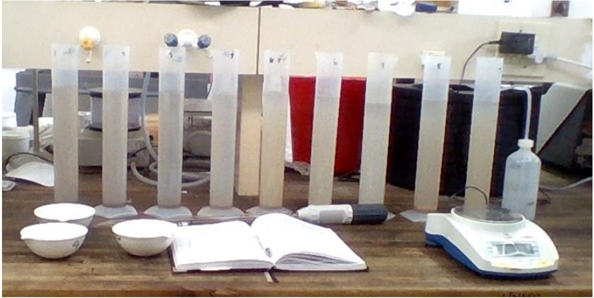
Figure 14. Materials used in the sedimentation method (500 ml cylinder, pipette, weighing balance and evaporating dishes).
