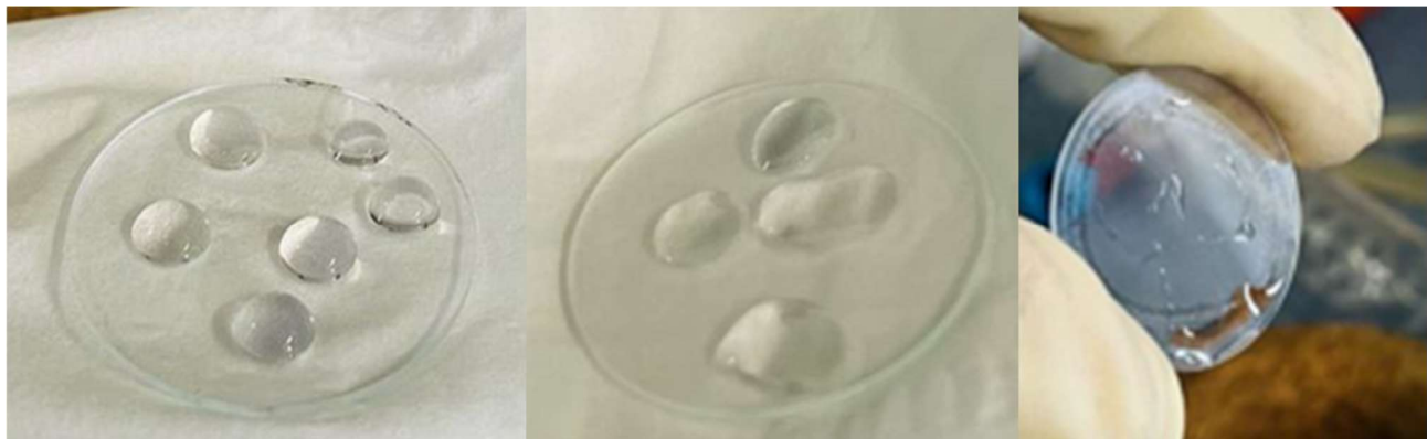
Figure 38 Assessing the hydrophobicity of the fabricated porous silica coatings with the glass on the left and two porous silica-coated glass on the right
