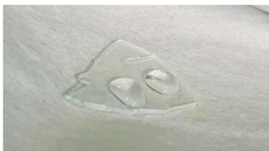
Figure 38 Assessing the hydrophobicity of the fabricated porous silica coatings with the glass on the left and two porous silica-coated glass on the right
