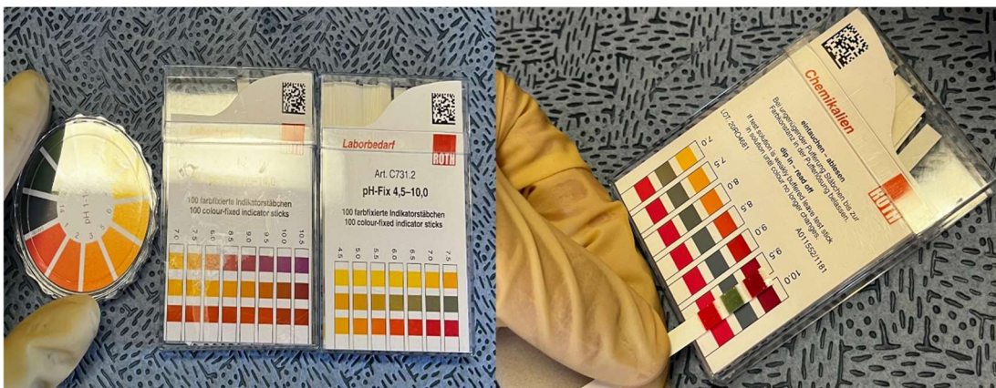
Figure 6 Three types of pH paper used in this study(left) and measuring the pH of a sol using a pH paper (right)
