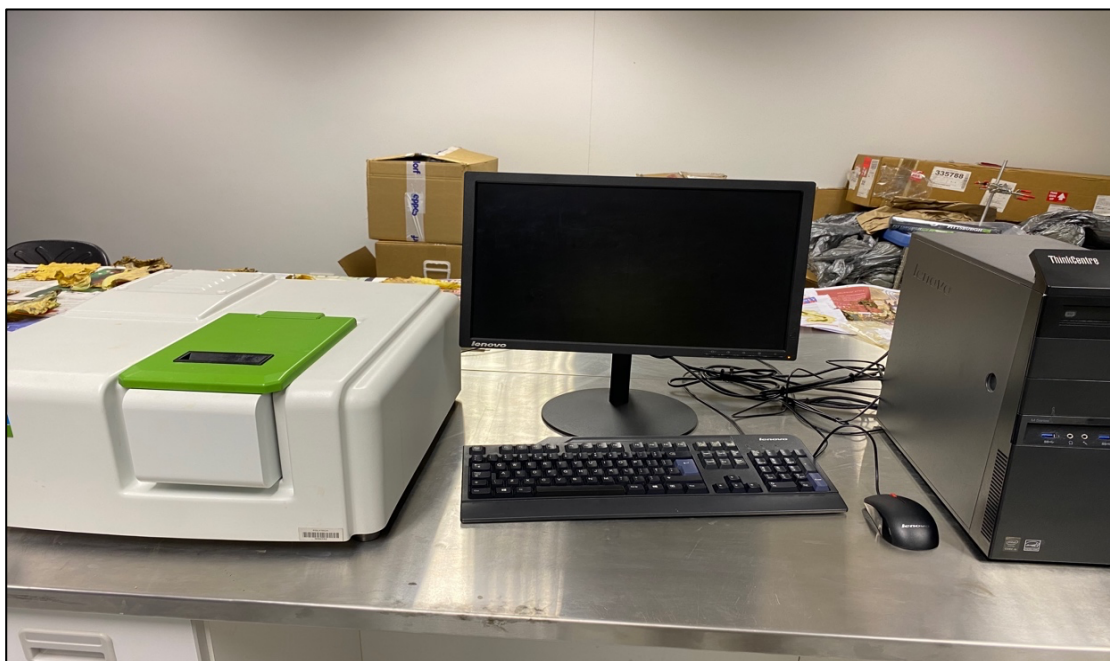
Figure 38: UV-Vis Spectroscopy used for absorbances of \text{Cu}^{2+} , MO and MB
