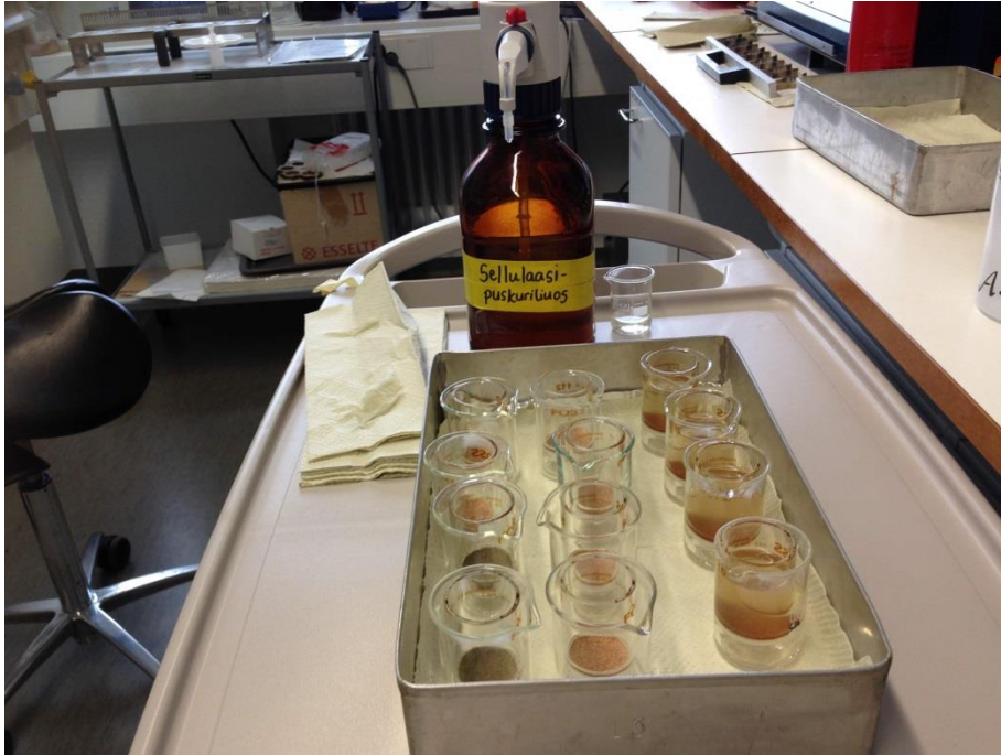
Figure 10.2 The process of the in vitro OMD, adding cellulose buffer solution to samples
