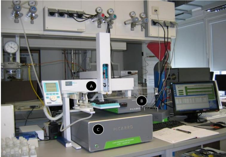
Figure 3.13: Major components of Isotope Ratio Infrared Spectrometer (L2120-i WS-CRDS) A: PAL auto-sampler, B: Picarro vaporizer, C: Picarro analyzer.
