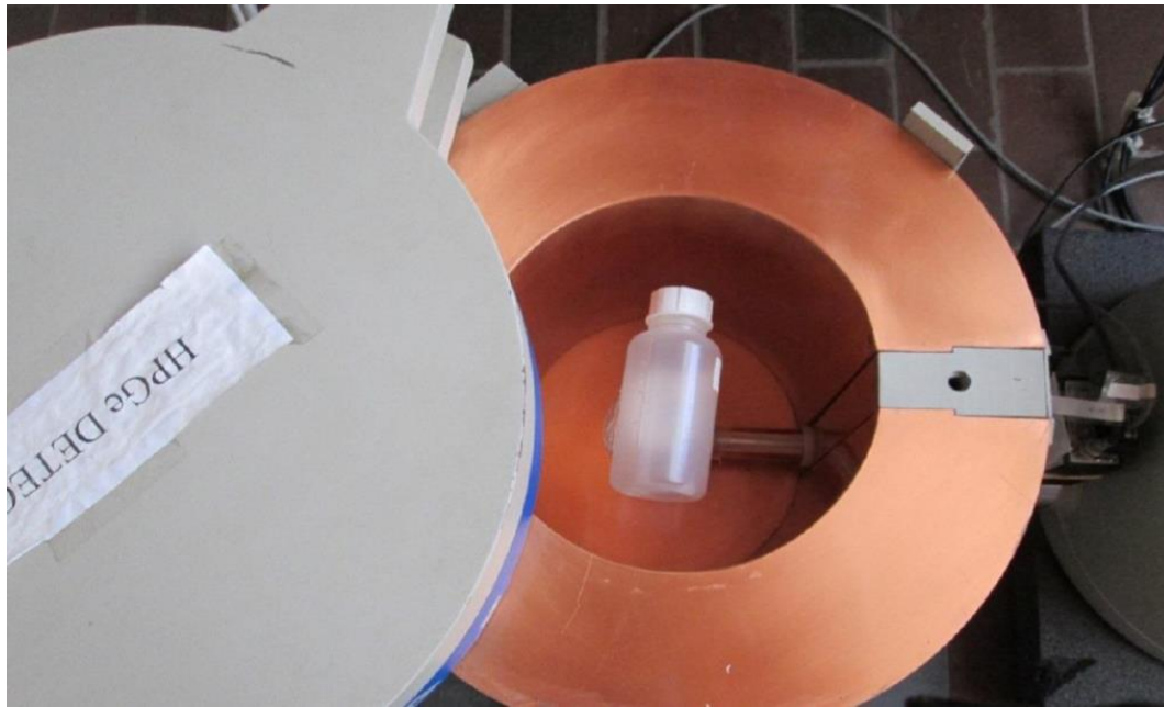
Figure 3.6. HPGe Detector with empty bottle ready for background counting [14]
