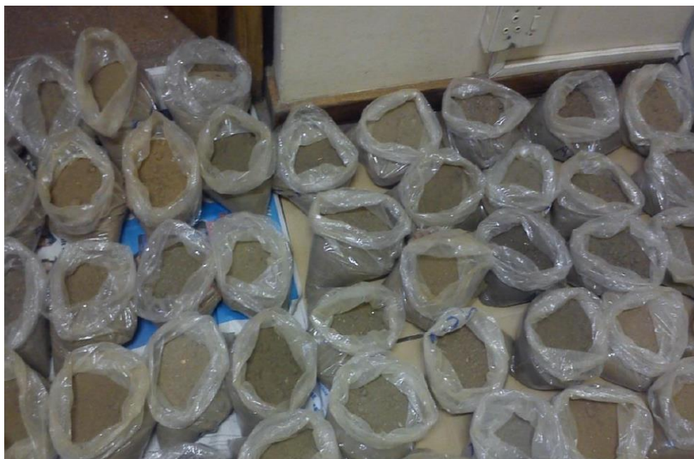
Figure 3.17 Drying of soil samples
