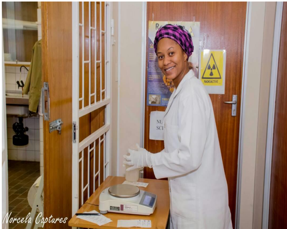
Figure 3.16. Determination of the weight of a soil sample using an electronic scale.
