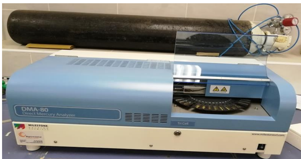
Figure 3.7: The DMA-80 milestone instrument used for total Hg quantification
