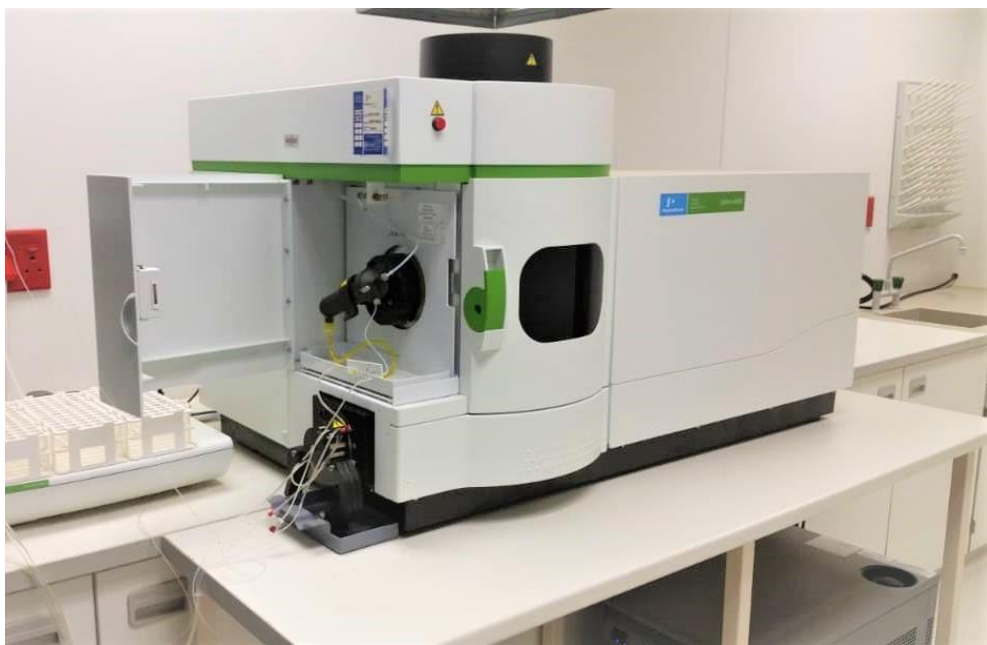
Figure 3.9: Inductively Coupled Plasma Optical Emission Spectrophotometer, ICPOES (Optima 8000, Perkin Elmer)
