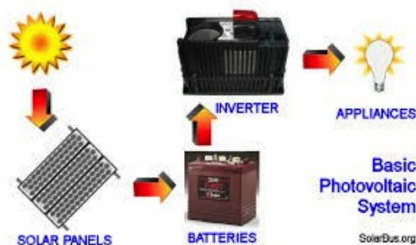
Figure 4: Schematic diagram of the basic solar system. Source: solarflux.org
