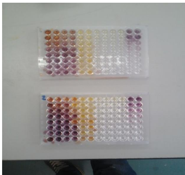
Fig 12: An image of 96 well plates loaded with sample, DMSO and DPPH before measuring the absorbance at 512nm.
