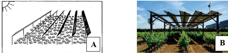
Figure 2.2: Sketch of the agrivoltaic idea in 1981 by Prof Goetzberger et al (A) [20]. Implementation of the agrivoltaic idea in real life systems (B) [12]
