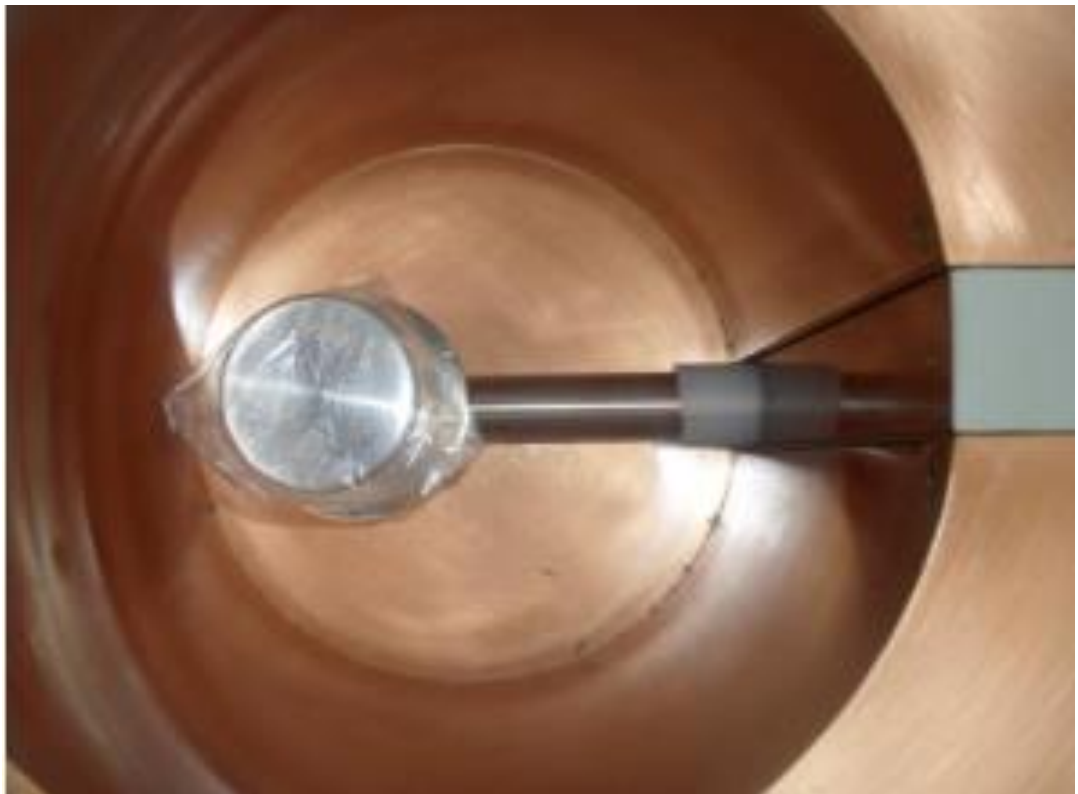
Figure 3.6: HPGe detector in a Lead shield
