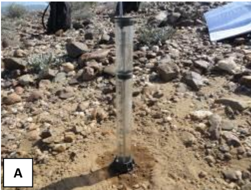
Figure 6. Picture A illustrates the set-up of mini-disc infiltrometer in the natural habitat and picture B demonstrates how the measurement of water infiltration rate was carried out in the field at Sendelingsdrif.
