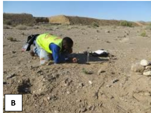
Figure 6. Picture A illustrates the set-up of mini-disc infiltrometer in the natural habitat and picture B demonstrates how the measurement of water infiltration rate was carried out in the field at Sendelingsdrif.
