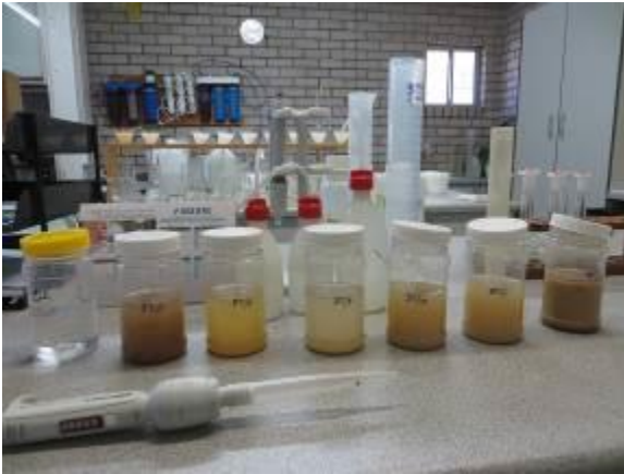
Figure 7. A photograph showing the bottles and the pipette that were used to determine the texture of soil samples at Analytical Laboratory Services in Windhoek.
