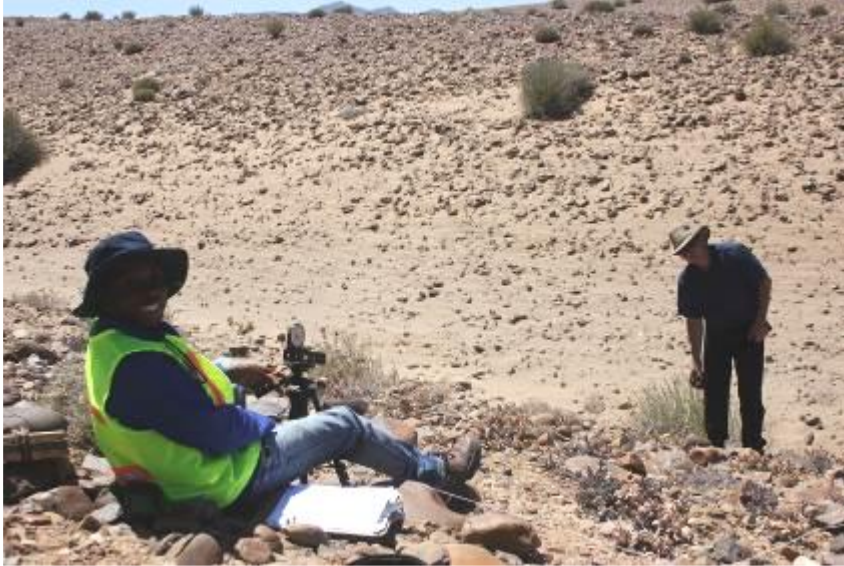
Figure 4. Using a clinometer to determine the slope angle for a survey plot at Sendelingsdrif diamond mine.
