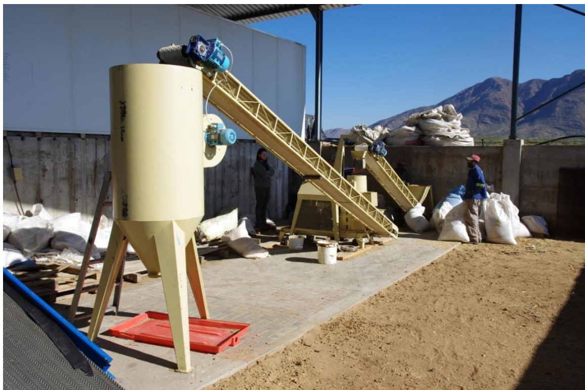
The picture on the left shows a pelletizer machine set up and on the right bush feed pellets
