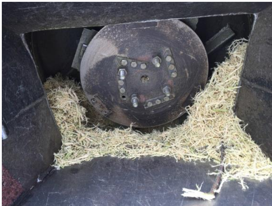
Appendix 27: Chipped bush feed passing through a hammer mill
