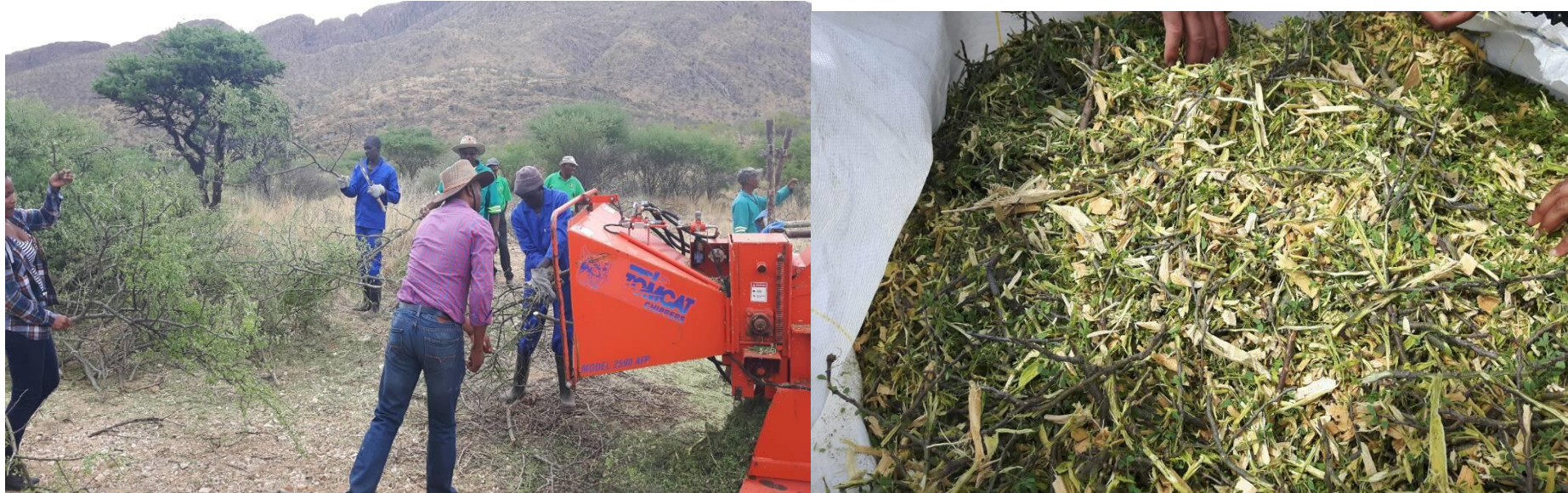
Manual harvesting of Senegalia mellifera bush and feeding in the wood chipper machine on the left picture and Wood chips from the chipper on the right
