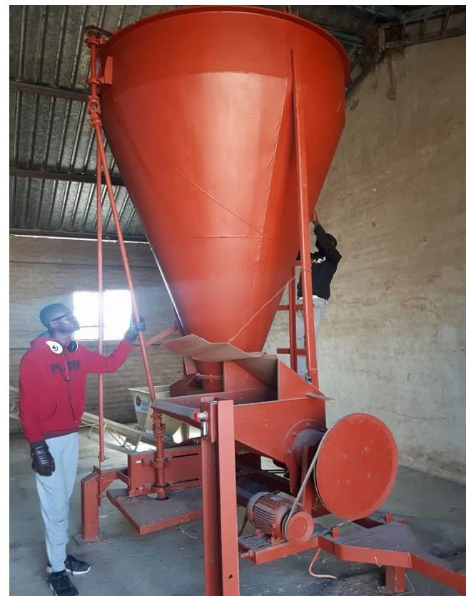
The picture on the left shows a hammer mill wheel with milled bush and on the right a mixer that is used to mix the ingredients with milled bush
