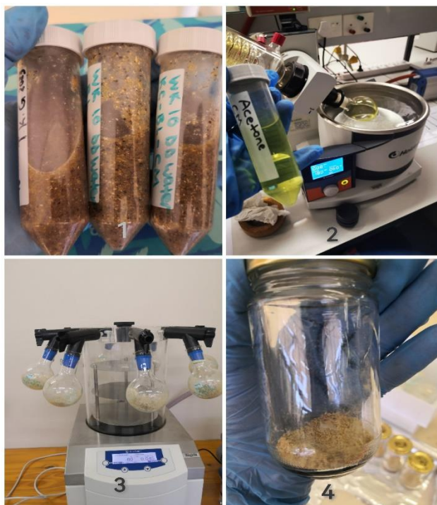
Figure 4.2: Extraction of okra pod extracts using different solvents (image 1) and the use of rotary evaporation (image 2) and freeze-drying (image 3) techniques to concentrate the extracts (image 4) for bioactive compounds analysis and antimicrobial testing.
