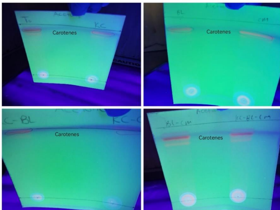
Figure 4.13: TLC results for okra pod extracts that were extracted with acetone for the eight different treatments (T 0 , KC, BL, CM, KC-BL, KC-CM, BL-CM and KC-BL-CM).
